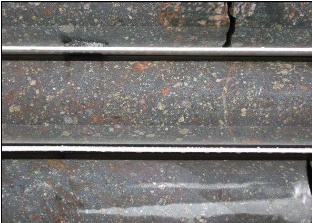
Figure 5. Photo of typical hematite matrix-rich mineralised core from VUD 007. Hematite is grey, sulphides (pyrite and chalcopyrite) are white/pale yellow. Width of photo about 15cm.
