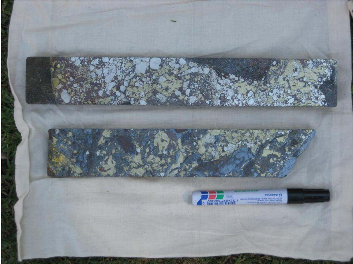
Figure 4. Cut drill core samples showing some of the higher grade chalcopyrite-pyrite mineralisation in VUD 003. Chalcopyrite is distinct yellow, and pyrite is white. Upper sample from 0.34m interval at 5.9% Cu, 2.23g/t Au; lower sample 0.75m at 4.4% Cu, 1.34g/t Au, 0.6kg/t U_3O_8 .
