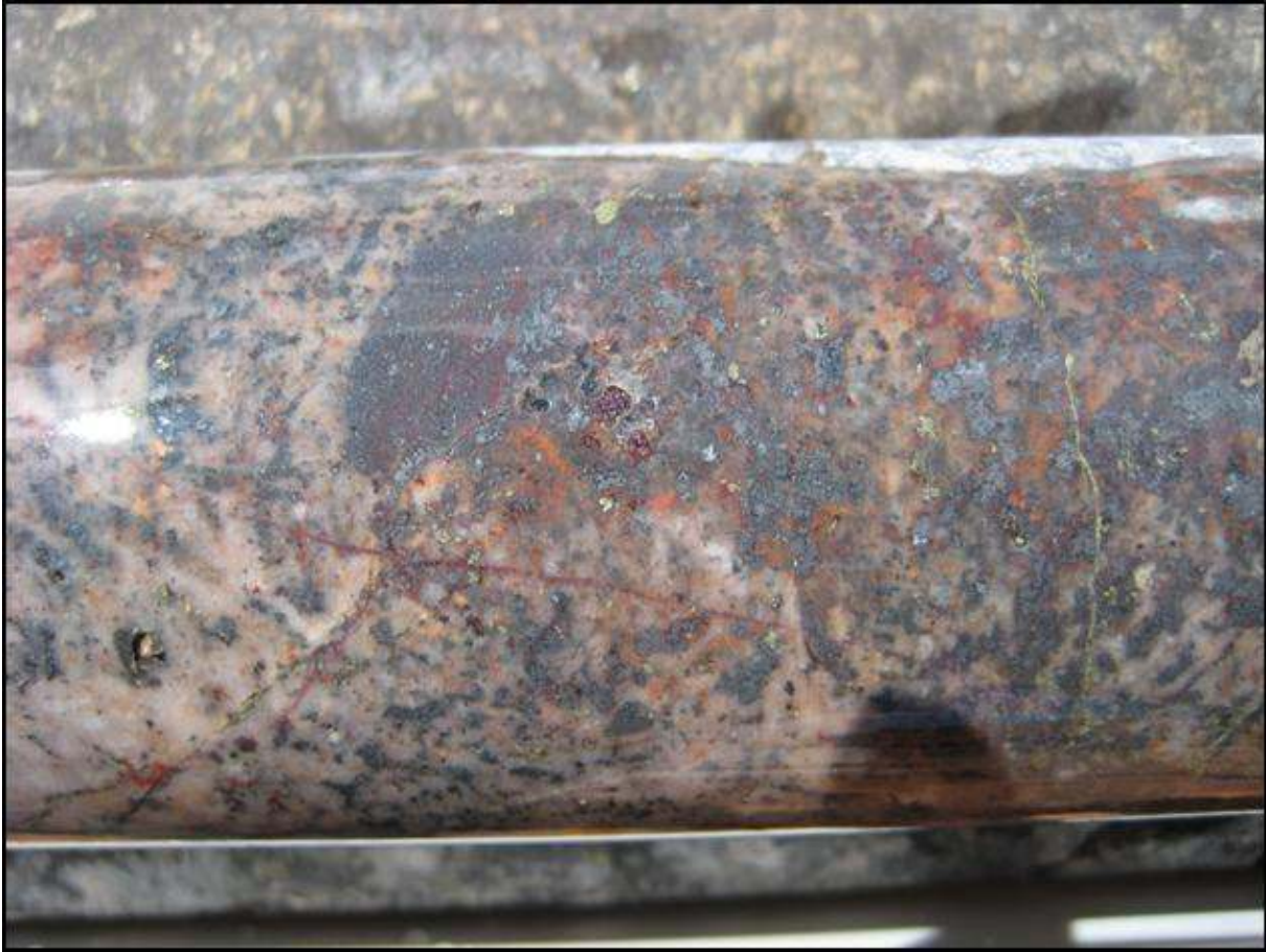
Figure 6. Close up photo of core from VUD 008, showing extreme silica (quartz) alteration (white-cream), hematite (steely grey) and disseminated bornite (purple, near centre of photo). Width of photo is about 15cm.
