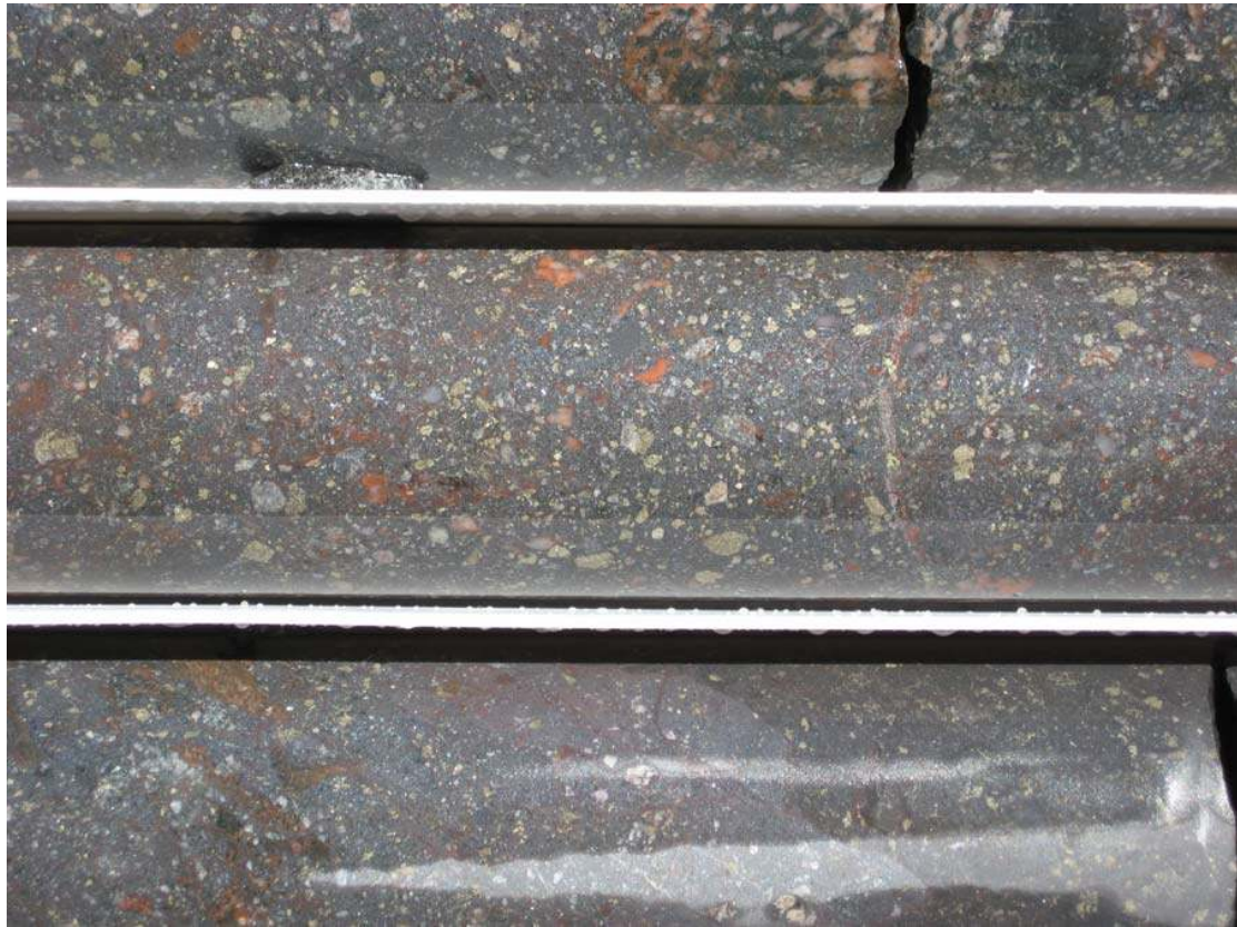
Figure 3: Close-up photo of hematite breccia from VUD 7. Hematite is dark grey and chalcopyrite is the yellow mineral prominent in the upper core segment. The other minerals are pyrite, carbonate (probably siderite), quartz and feldspar. (NQ Core – approx. 50mm diameter).
