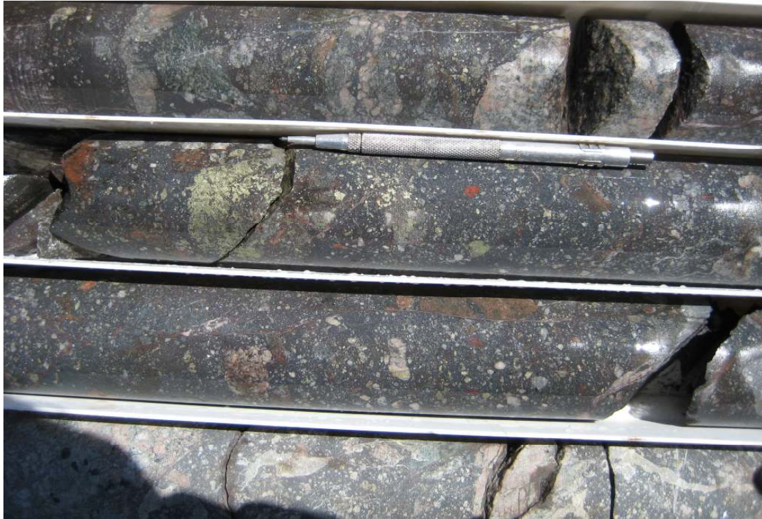
Figure 2: Close-up photo of typical hematite breccia from VUD 7. Hematite is dark grey, sulphides (pyrite and chalcopyrite) are yellow/silverish and the other minerals are carbonate (probably siderite), quartz and feldspar. (NQ Core – approx. 50mm diameter).
