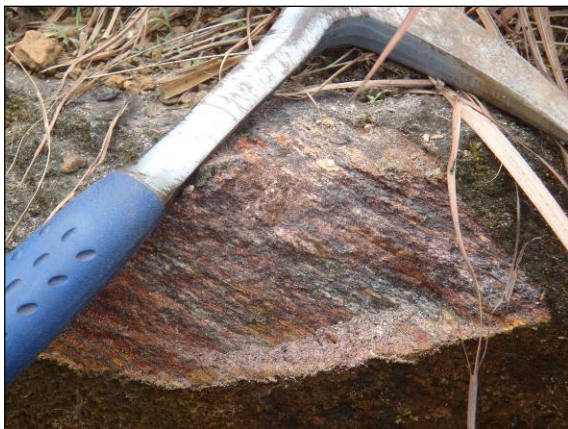
Left: Medium-coarse grained, laminated quartz-magnetite iron formation (sample MC1001). Right: weathered variety of similar rock type crushed by hand forming soft, friable quartz-magnetite sands easily beneficiated by magnet pen (sample MC1003).
