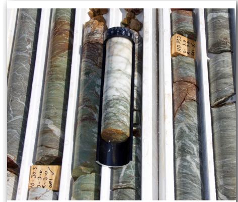
Fig 1. Portion of HQ diameter drill core recovered during drilling from McPhees prospect, Talga Talga gold project.
