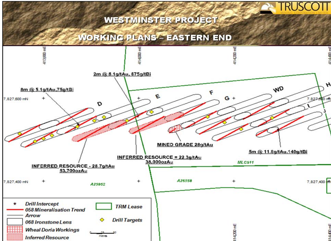
Figure 2: Westminster Project – Working Plans – Eastern End
