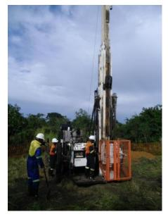
Initial drilling of 30 diamond drill-holes for 1,000 metres is designed to outline manganese veins around the small pit and test for extensions along strike to the south-west.
