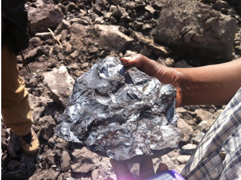
Manganese Ore from the Chowa Open Pit - dark coloured, highly brilliant, very low Iron characterizing the type of material on site.
