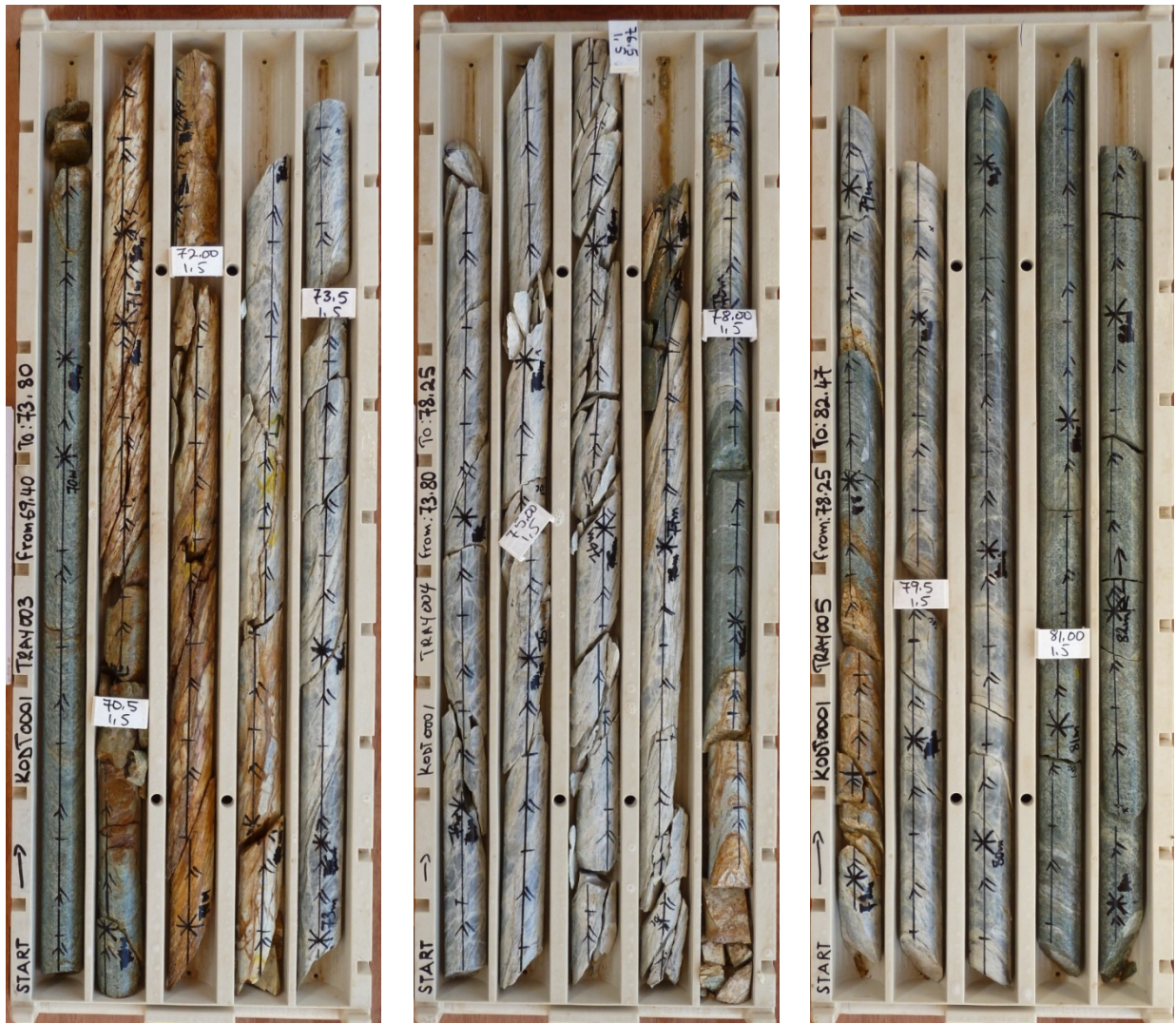
Photo 1:- Core from KODT001 (extension of KORC002) 69.40 – 82.47m Drill core exhibiting strong quartz veining-silica-carbonate-pyrite alteration – note assays pending
