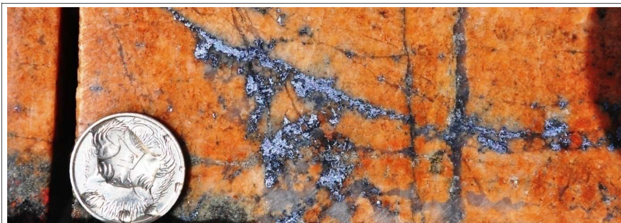
Drill core showing molybdenite veins in altered porphyry
