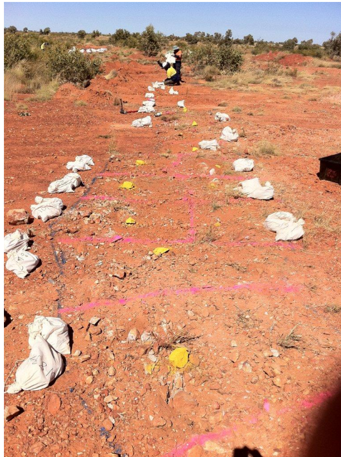
Figure 4. Gridded and sampled vein (pink lines represent grid boundaries of vein samples).
