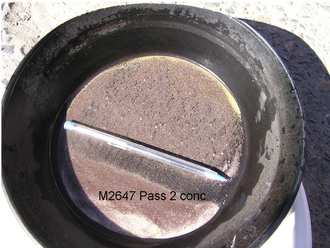
Figure 1. Gold Pan concentrates from Knelson Concentrator test work. Top = First Pass concentrate from 220 micron grind. Bottom = second pass concentrate from 113 micron grind.
