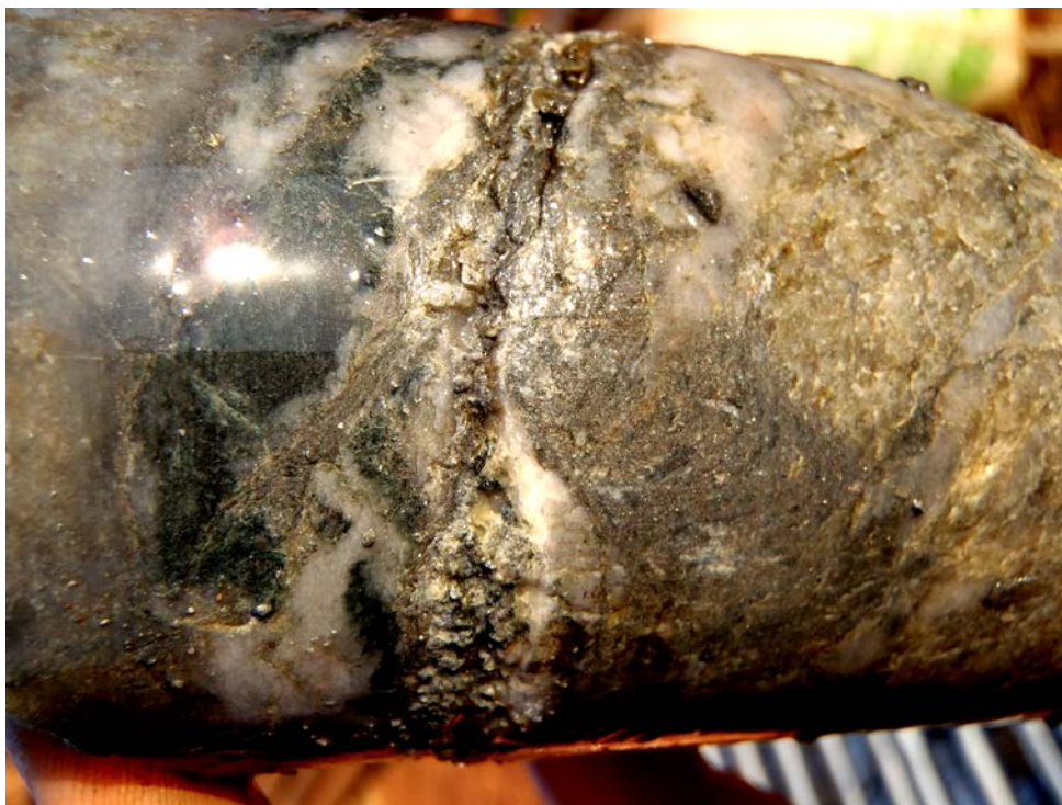
Photograph. Core sample from BCRD100006 in the Caribbean Zone showing highly silicified fault zone with quartz, sulphide and chlorite / clay alteration. Field of view ~10cm.
