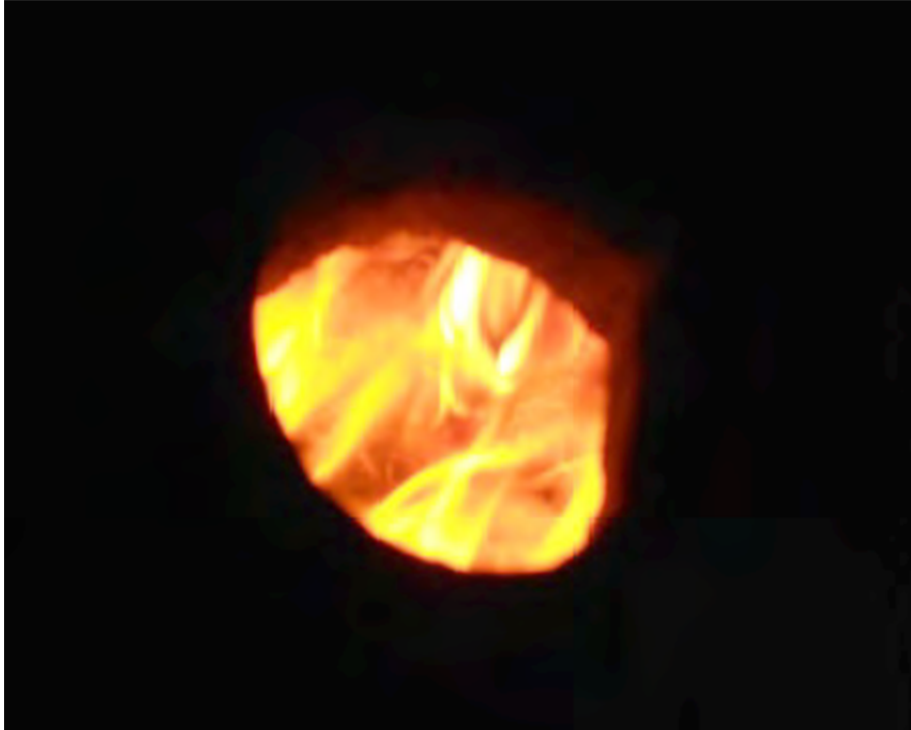
Diagram 3. Inspection peephole showing Sese coal igniting under arch
