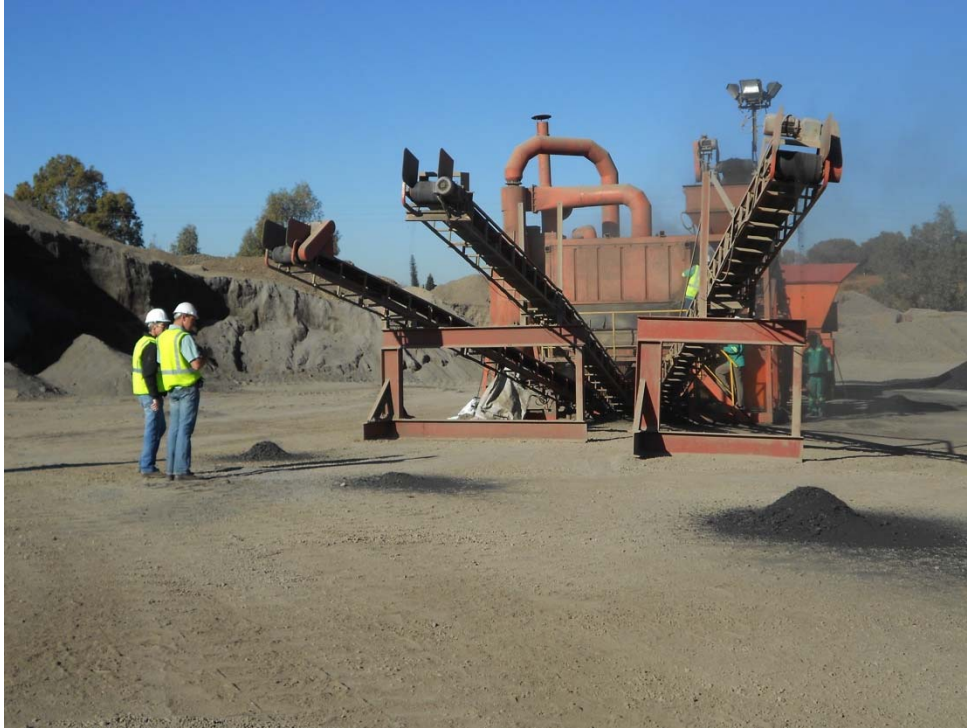
Diagram 1. Sese coal passing through Gecko Mineral Processing's pilot scale air-separator plant in South Africa
