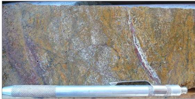
Figure 4: Photos of Oxidised Meta-Carbonatite Drilling Samples as per Sample EB-01
