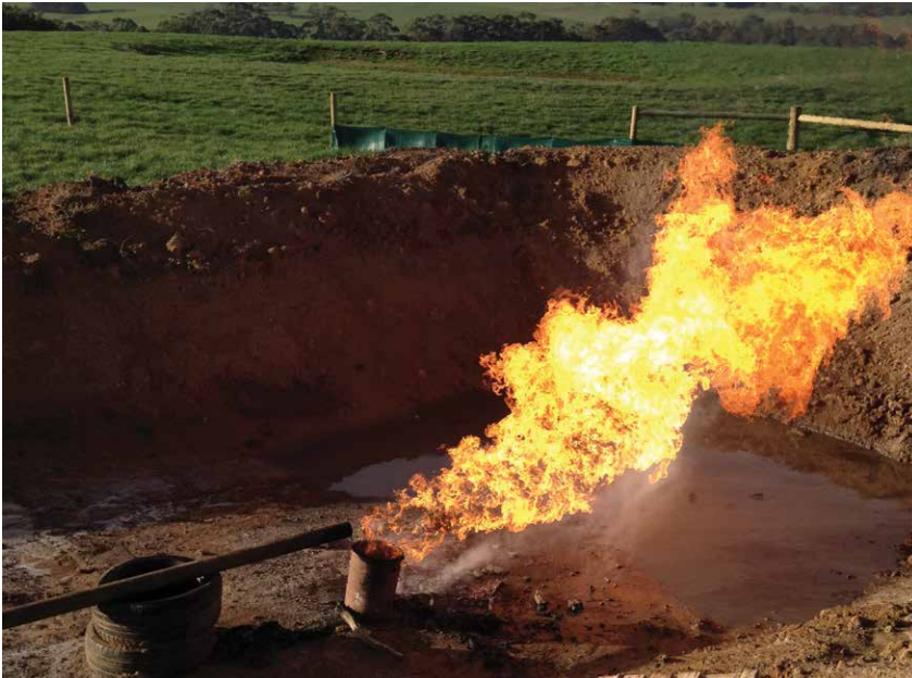
Figure 11 Gas and condensate flare from the Eumeralla Formation during the Moreys Drill Stem Test
