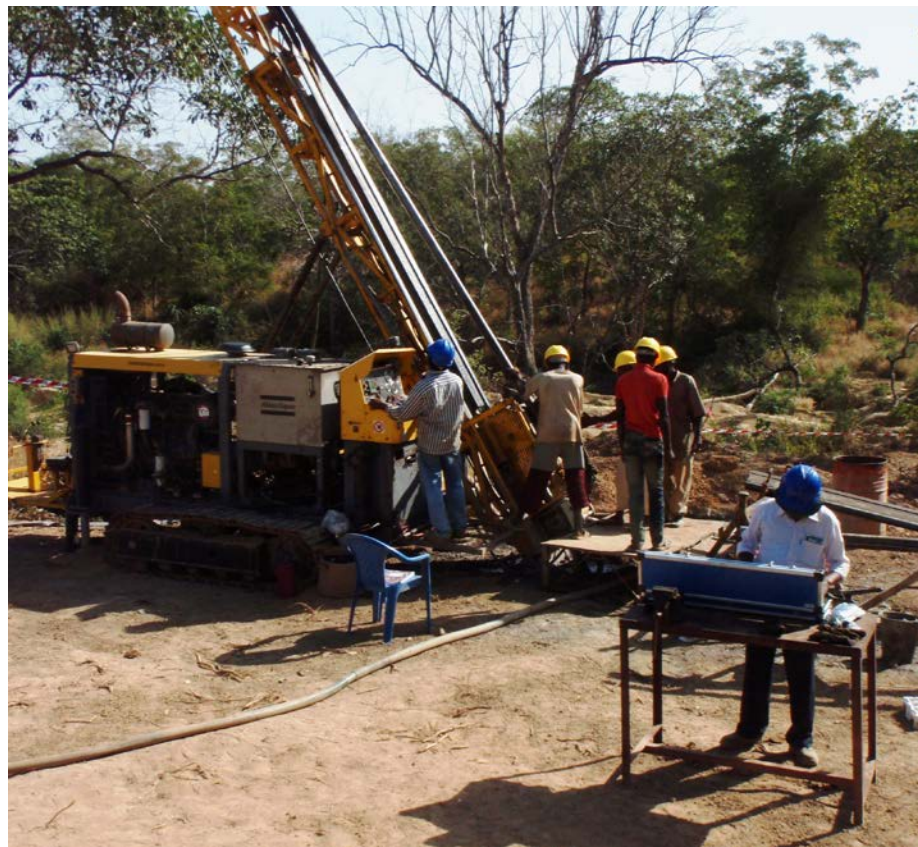
Diamond core drilling currently in progress at Yargarma (photo taken at hole YADD001)
