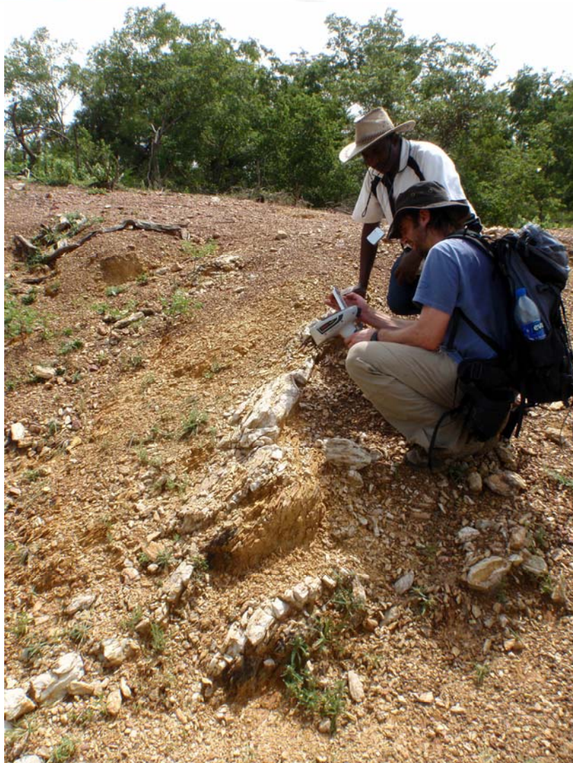
Figure 4: An example of the quartz veins observed across the Kasele project by the Company's exploration team during their recent field reconnaissance program. XRF analysis of this vein located within the S-02 target region returned elevated gold values. Australian Mines is proposing to include this target in its upcoming diamond core drilling program at Kasele.
