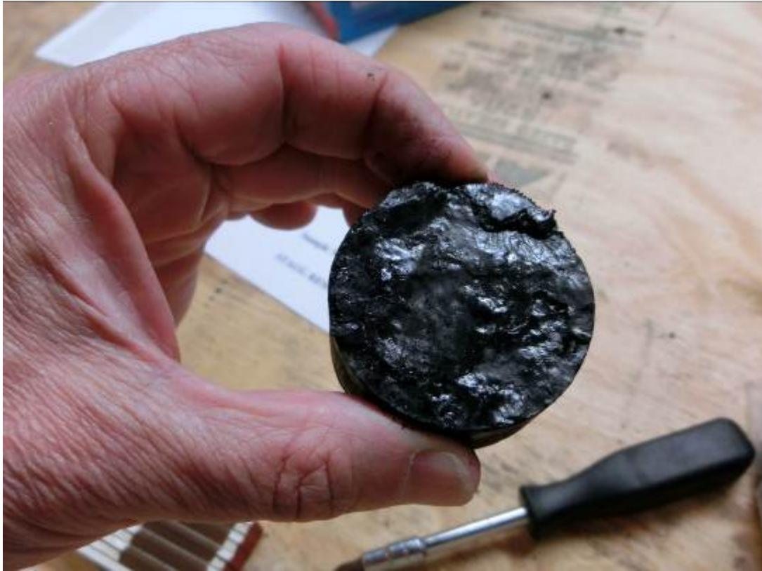
Figure 3. Sample of hard coking coal taken from core drilling on Coke Coal seam
