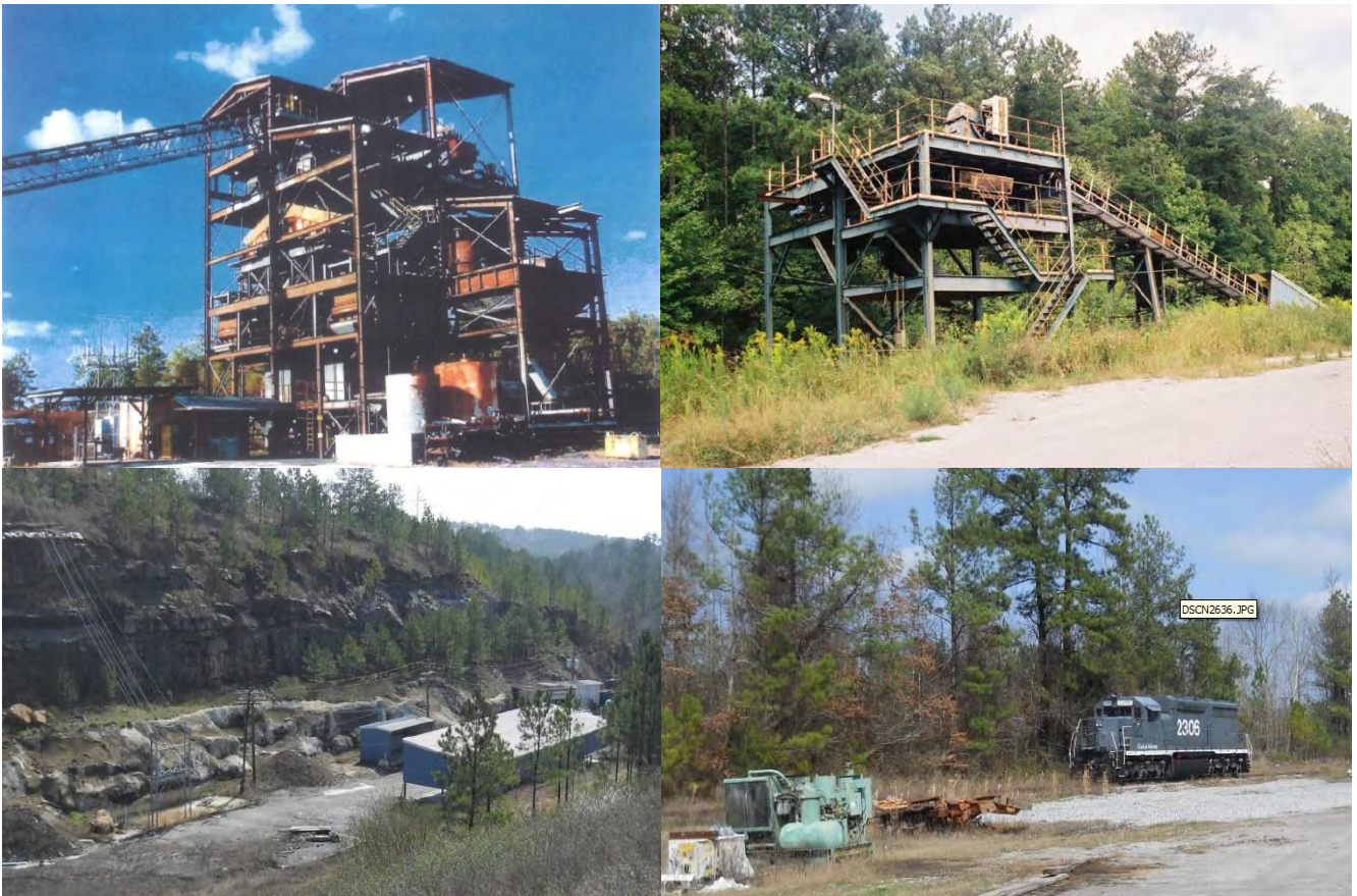
Figure 7 Sample of infrastructure owned by Kodiak; top left - 300tph wash plant, top right - the rail load out facility, bottom left - mine portal and mains power, bottom right – rail spur and locomotive.
