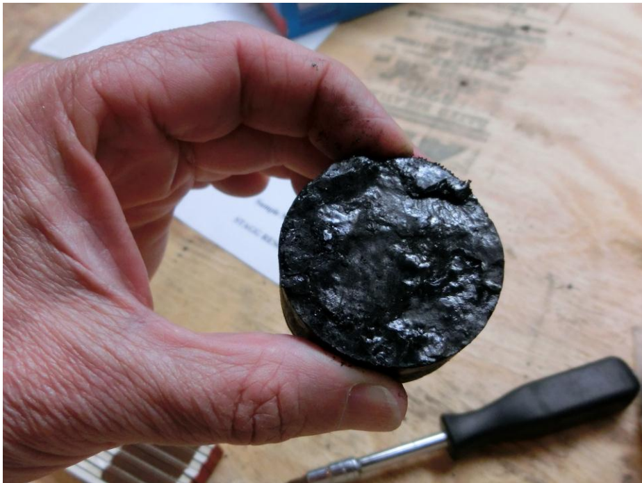
Figure 3. Sample of coking coal taken from core drilling on Coke Coal seam.
