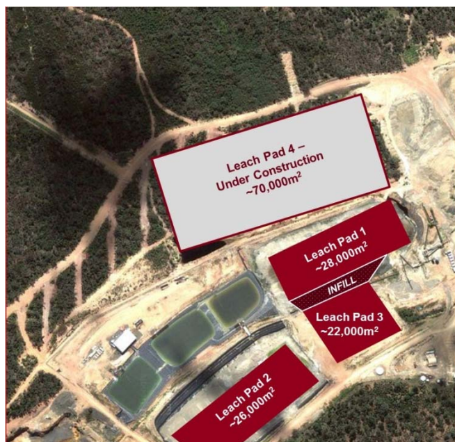
Figure 1: Aerial view of Texas Operations showing Leach Pad configuration and increasing area under irrigation
