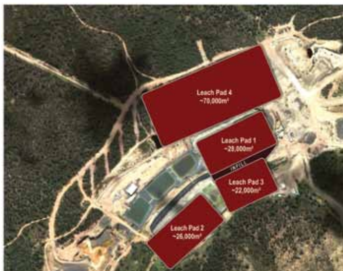
Figure 1. Current Leach Pad Configuration
