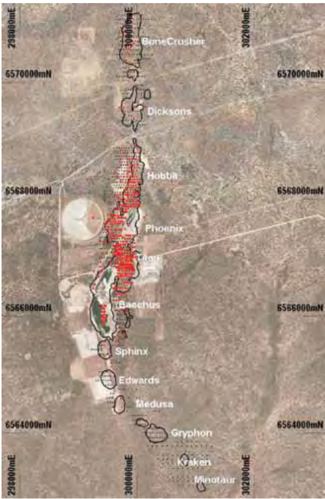
Figure 5.7. Drill location plan showing potential optimised pit outlines for the various resource target areas along the Bullabulling structural trend (red filled drill collars are completed holes).
