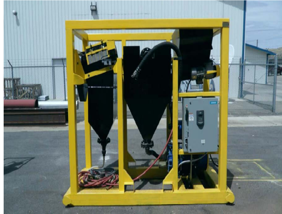
Pilot-scale Ablation unit that processes ~0.5 tonnes/hour. This technology is being scaled up to units that can process ~20 tonnes/hour.
