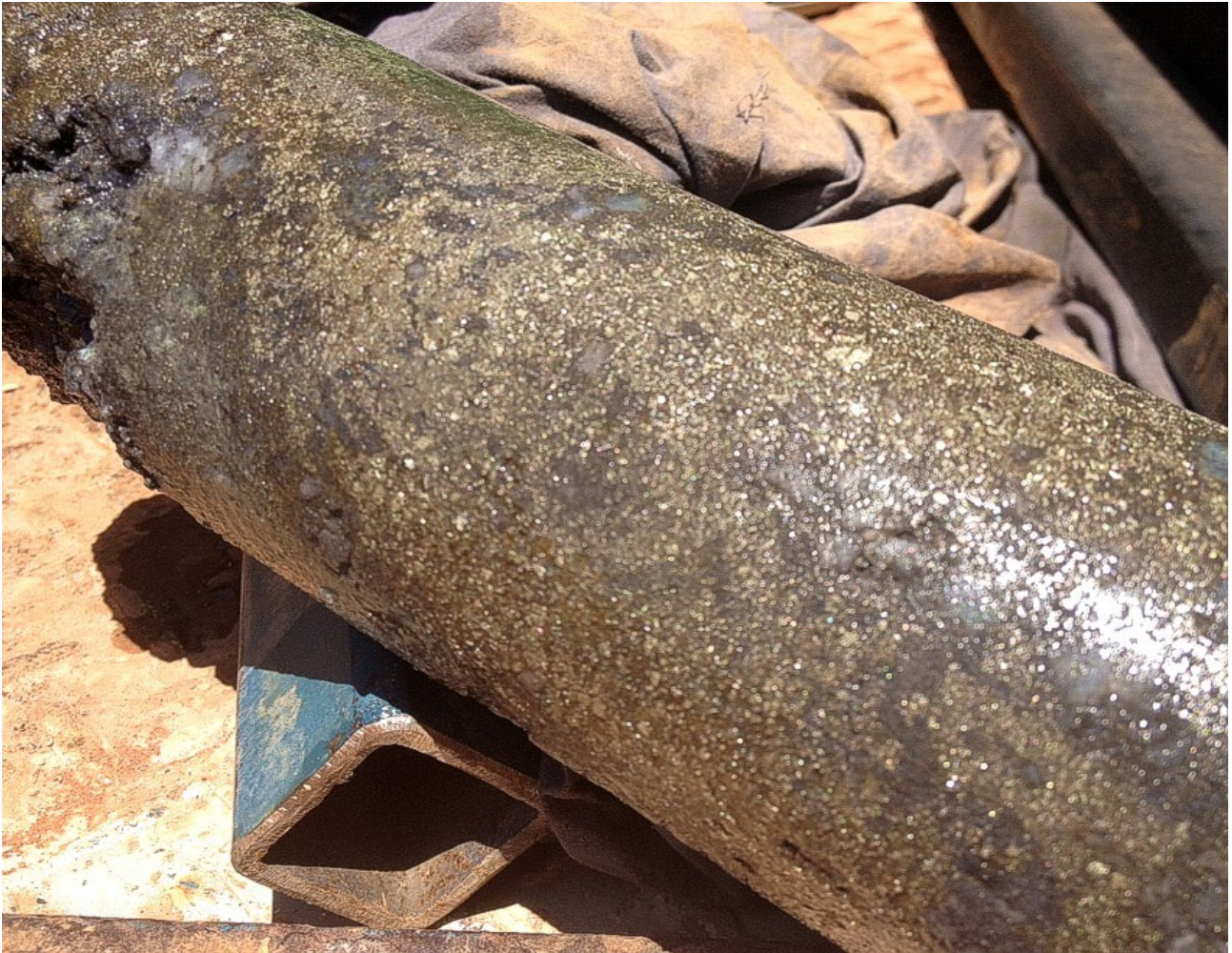
Figure 9: Example of high-grade drill core intersected in DODDH448 at Fairfield at approx. 83m. Massive and semi-massive chalcopyrite and pyrite and minor chalcocite and bornite. Chalcocite contains 79.9% copper metal, chalcopyrite contains 34.6% copper metal, bornite contains 63.3% copper metal and cobalt is usually associated with pyrite at Fairfield.
