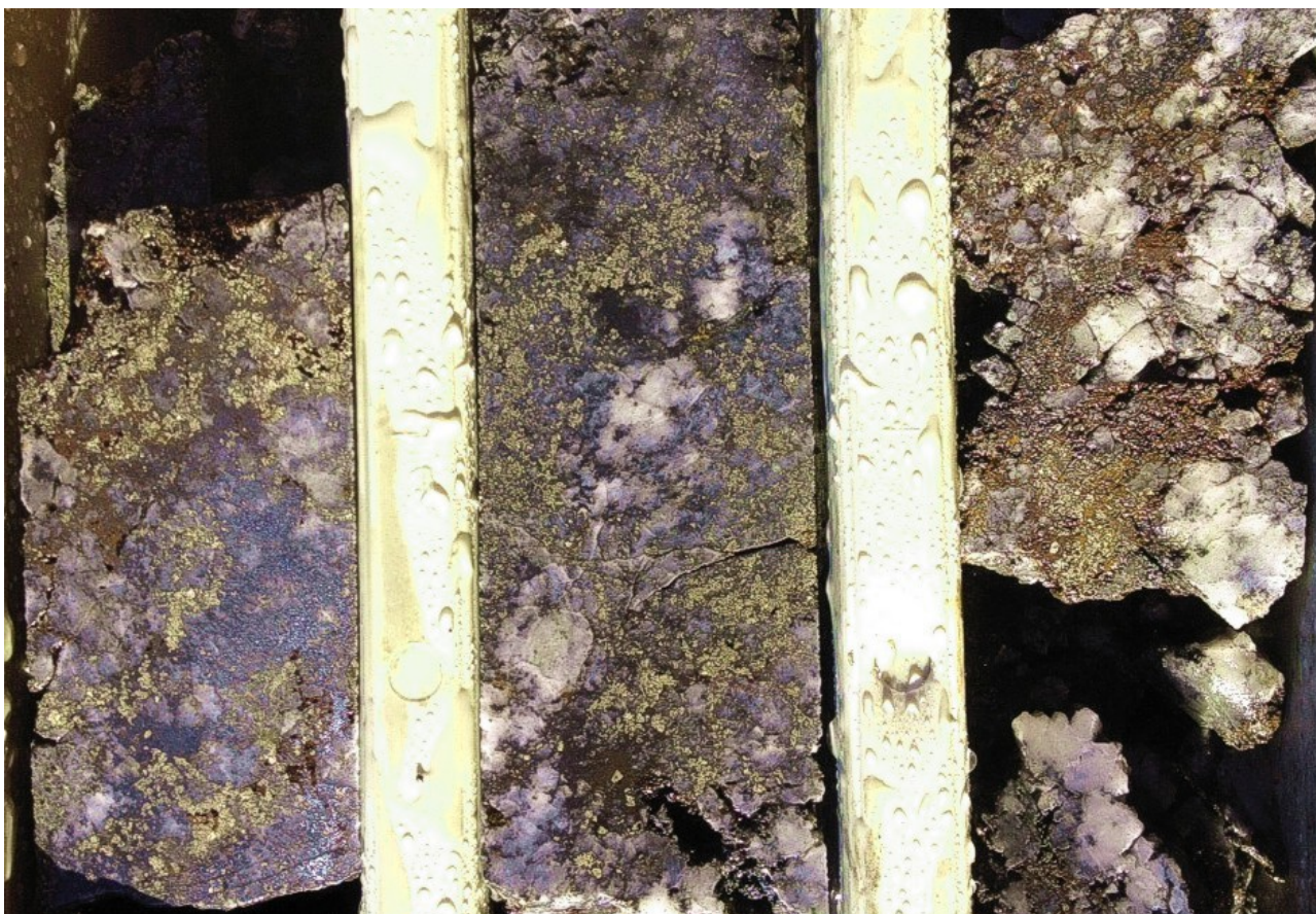
Figure 2: Example of high-grade drill core intersected in DODDH447 at Fairfield (approximately 84m - 86.4m). Highly-weathered semi-massive chalcocite and chalcopyrite (chalcocite contains 79.9% copper metal, chalcopyrite contains 34.6% copper metal), bornite (bornite contains 63.3% copper metal) and pyrite (cobalt is associated with pyrite at Fairfield)
