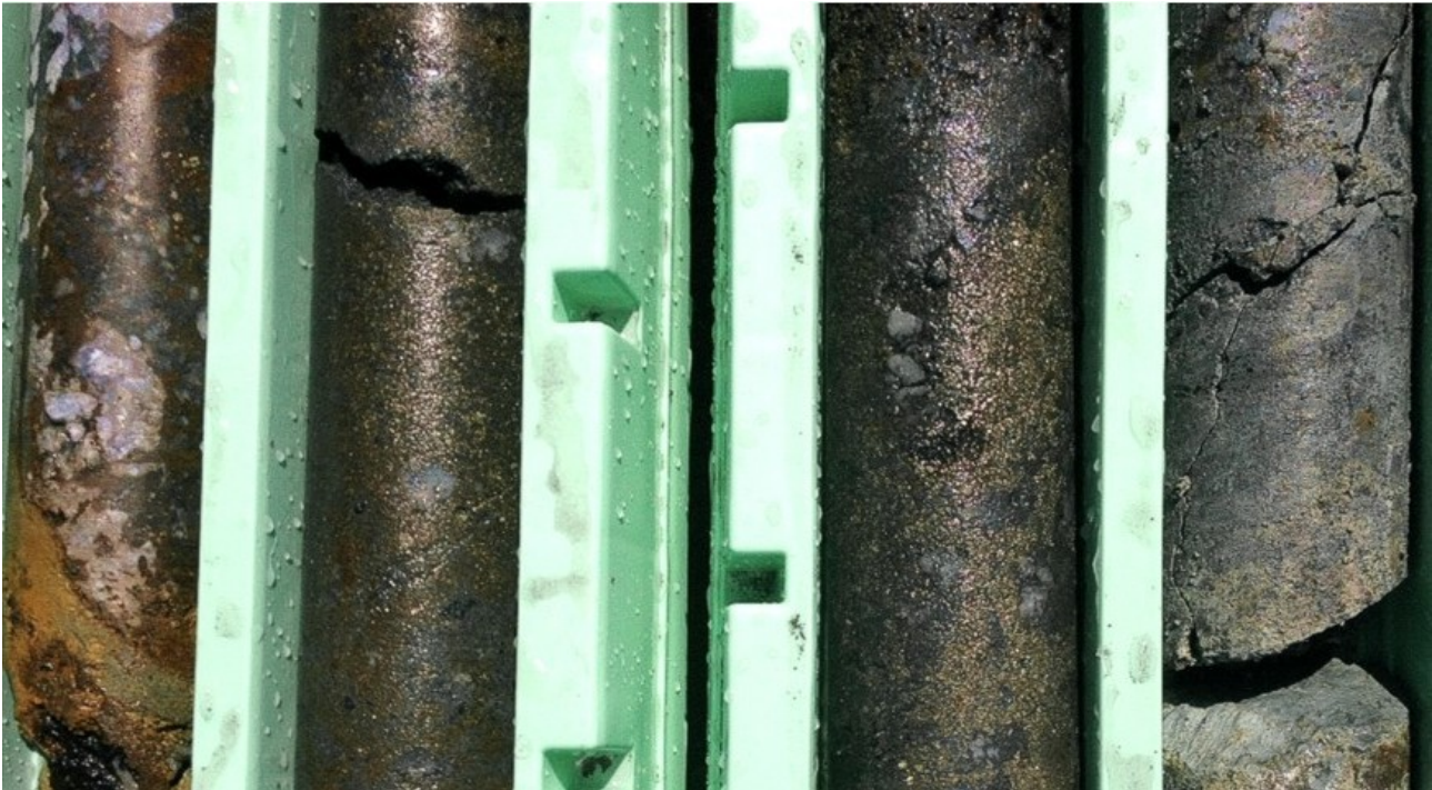
Figure 6: Example of drill core from approximately 81m - 84m in diamond drill core DODH448. Massive and semi-massive chalcocite, chalcopyrite and pyrite and minor bornite in highly-weathered breccia matrix - hole currently still drilling in mineralisation at 97m (assays awaited). Chalcocite contains 79.9% copper metal, chalcopyrite contains 34.6% copper metal, bornite contains 63.3% copper metal and cobalt is usually associated with pyrite at Fairfield.
