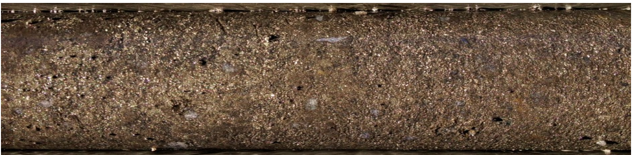
Figure 4: Example of high-grade drill core intersected in DODH446 at Fairfield (approximately 69m). Massive and semi-massive chalcocite and chalcocopyrite (chalcocite contains 79.9% copper metal, chalcocopyrite contains 34.6% copper metal).
