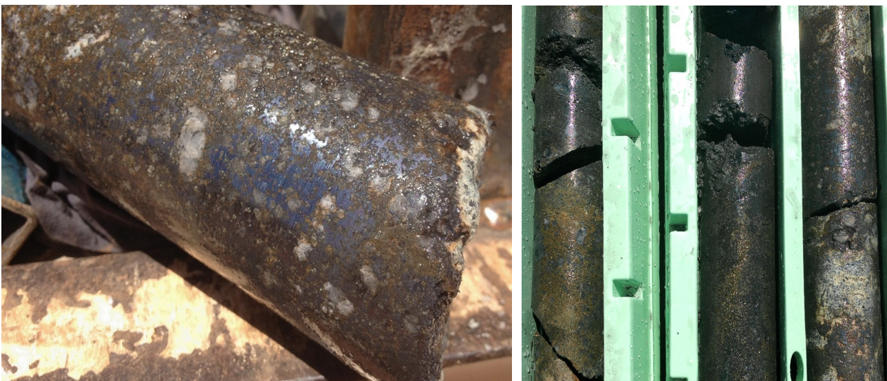
Figure 1: Example of high-grade drill core intersected in DODD448 at Fairfield. Massive and semi-massive chalcocite (chalcocite contains 79.9% copper metal), and minor chalcopyrite (chalcopyrite contains 34.6% copper metal), bornite (bornite contains 63.3% copper metal) and pyrite (cobalt is associated with pyrite at Fairfield). Left approx. 83m, right approx. 81-84m
