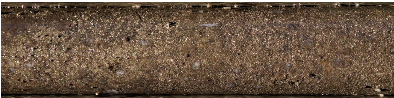
Figure 4: Example of high-grade drill core intersected in DODH446 at Fairfield (approximately 69m). Massive and semi-massive chalcocite and chalcopyrite (chalcocite contains 79.9% copper metal, chalcopyrite contains 34.6% copper metal).
