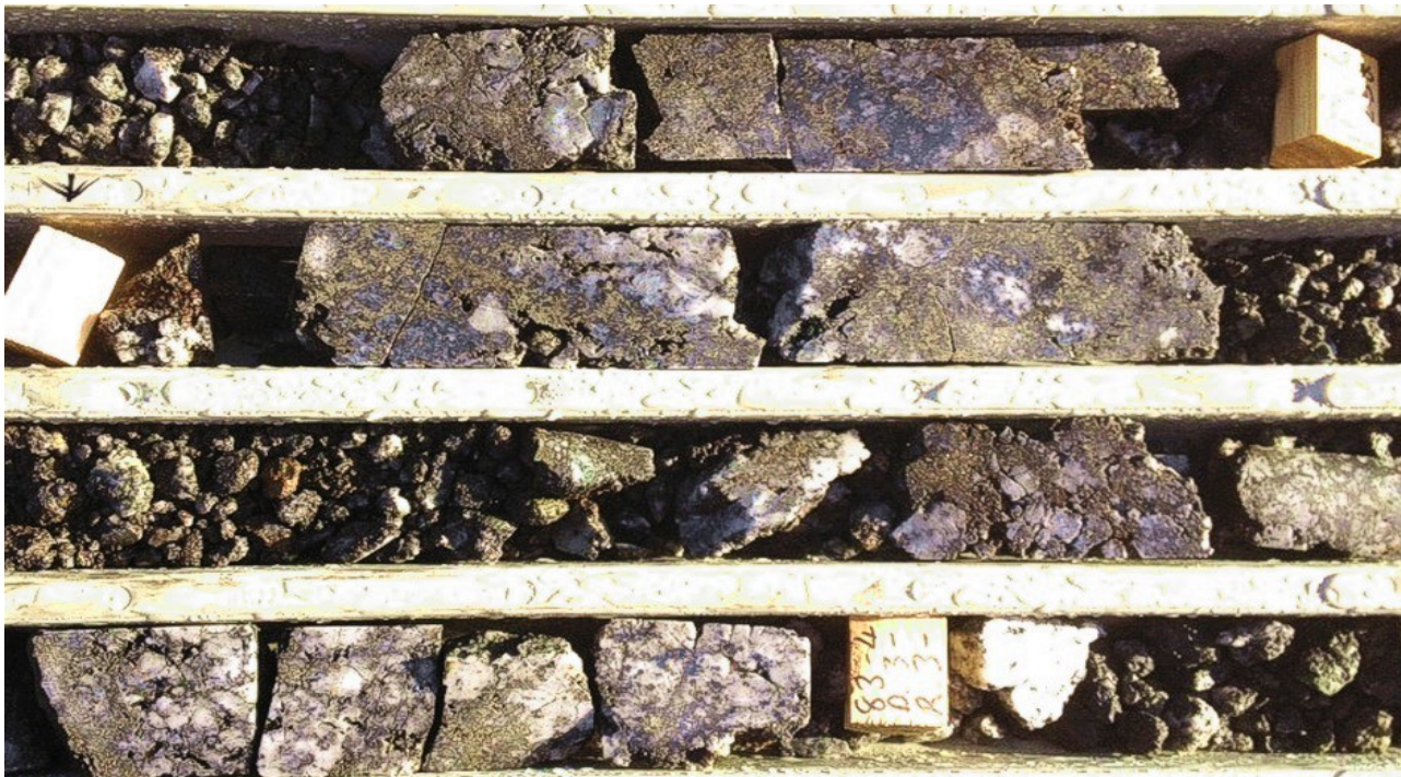
Figure 6: Example of drill core from approximately 83m - 87m in diamond drill core DODH447 which assayed 5m @ 9.92% CuEq (8.96% Cu, 1200ppm Co, Au pending) at Fairfield. Supergene chalcocite, chalcopyrite, bornite and pyrite in breccia matrix. Chalcocite contains 79.9% copper metal, chalcopyrite contains 34.6% copper metal, bornite contains 63.3% copper metal and cobalt is usually associated with pyrite at Fairfield.
