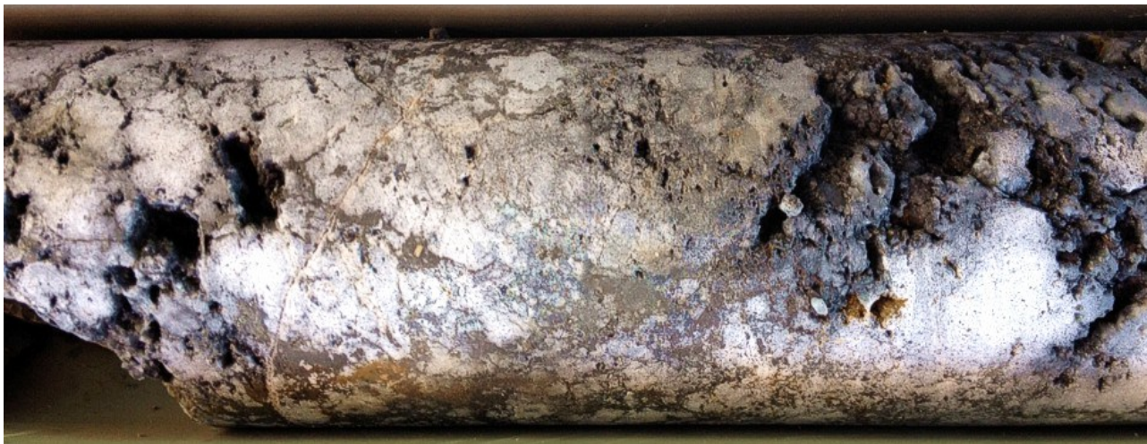
Figure 7: Example of drill core from approximately 83m in diamond drill hole DODH446 at Fairfield. Semi-massive chalcocite in highly-weathered quartz breccia (chalcocite contains 79.9% copper metal). Voids show traces of soft sooty chalcocite, thought to have been washed out via high-pressure drilling fluids often required when drilling through vuggy or highly porous matrix.
