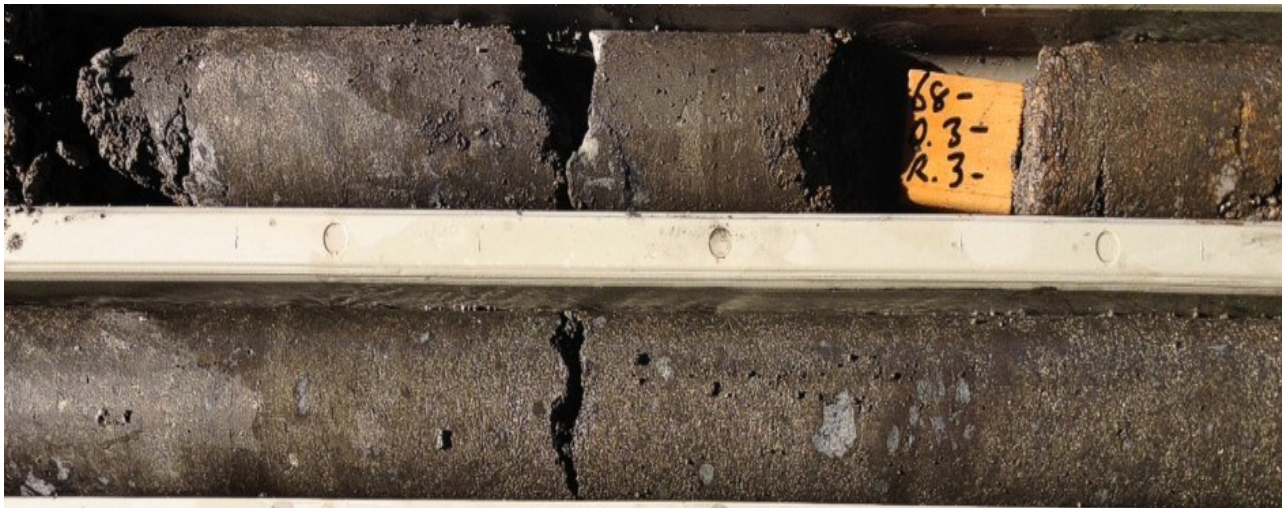
Figure 9: Example of high-grade drill core intersected in DODDH446 at Fairfield (approximately 68-69m). Massive and semi-massive chalcocite and chalcopyrite (chalcocite contains 79.9% copper metal, chalcopyrite contains 34.6% copper metal).
