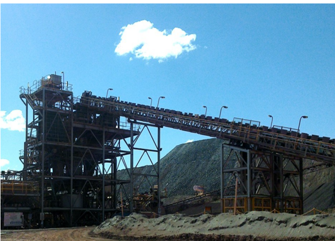
Figure 8: example of Rocklands scale (3mtpa), allmineral alljig® gravity plant at BHP's Whyalla Project, South Australia, manufactured by allmineral, Germany.
