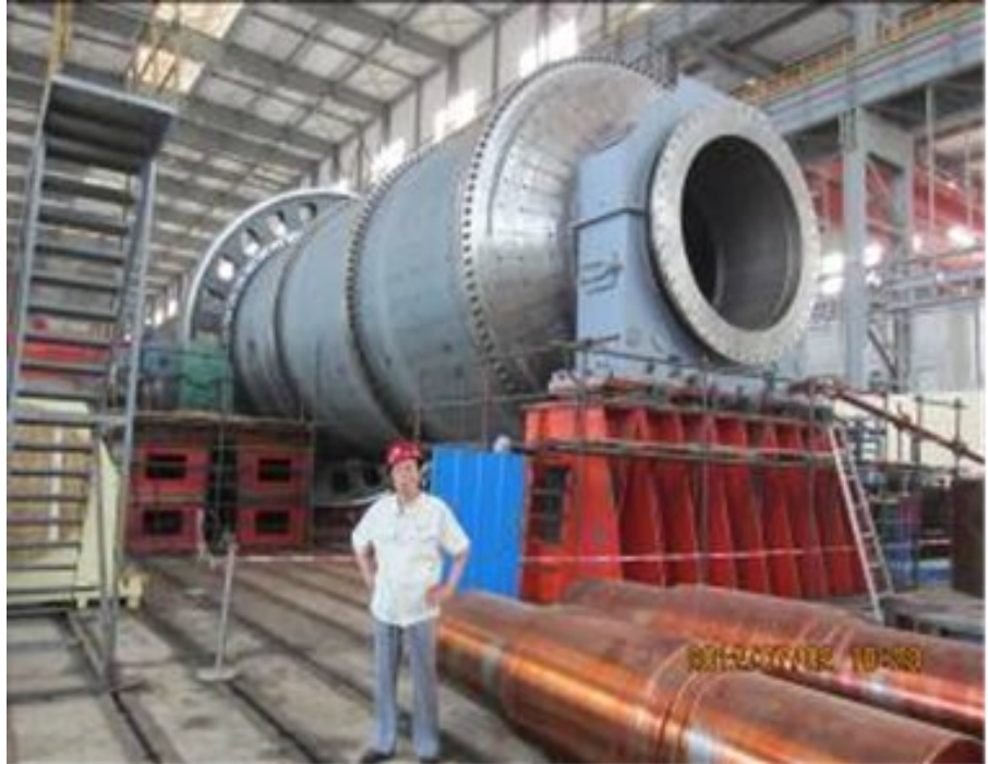
Figure 7: Smaller Ball mill being completed at Citics China facility
