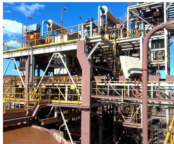
Figure 9: example of Rocklands scale (3mtpa), allmineral alljig® gravity plant at BHP's Whyalla project, South Australia - alljig's® to the left, spirals to the right
