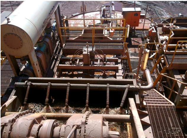
Figure 10: example of Rocklands scale (3mtpa), allmineral alljig® gravity plant at BHP's Whyalla Project, South Australia - alljig® Jig plant, foreground feed system
