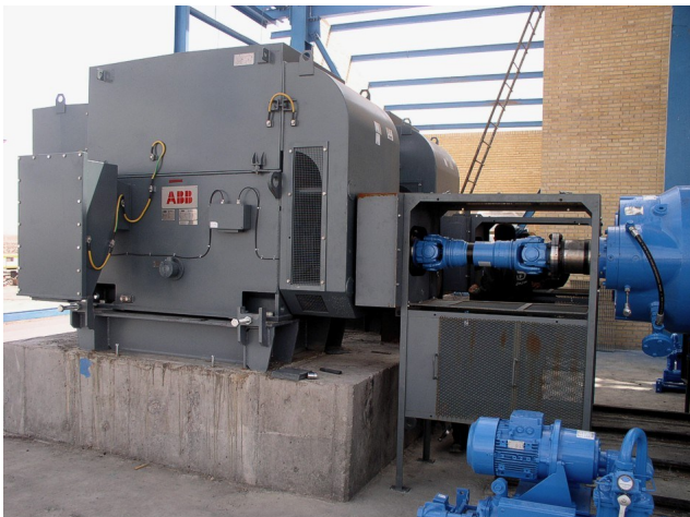
Figure 16: HPGR drive motor and driveshaft - recent HPGR installation by Polysius in the Middle East
