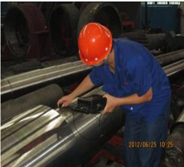
Figure 6: Testing of Shafts - CuDeco's primary Ball Mill
