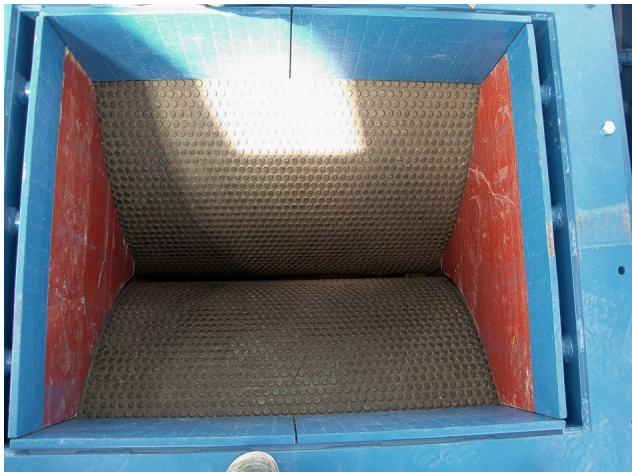
Figure 14: HPGR showing studded grinding rolls in position - recent HPGR installation by Polysius in the Middle East
