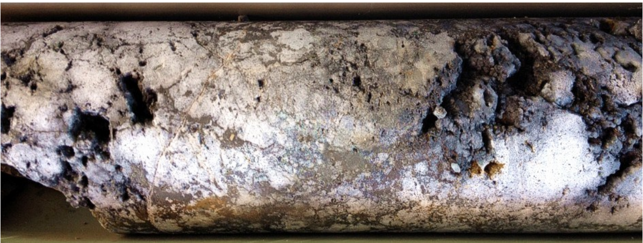
Figure 6: Example of drill core from approximately 83m in diamond drill hole DODH446 at Fairfield. Semi-massive chalcocite in highly-weathered quartz breccia (chalcocite contains 79.9% copper metal). Voids show traces of soft sooty chalcocite, thought to have been
