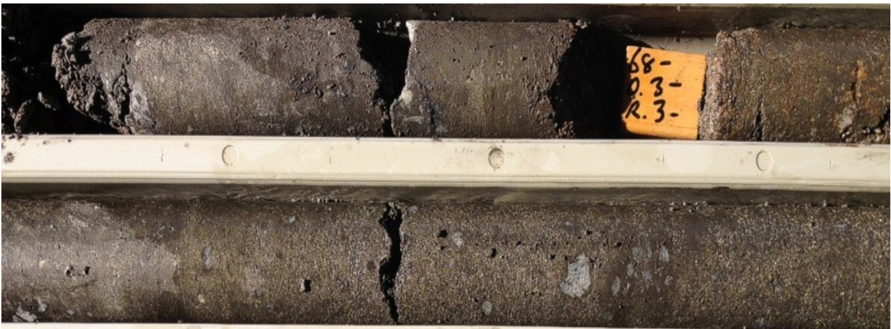
Figure 3: Example of high-grade drill core currently being intersected in DODH446 at Fairfield (approximately 68-69m). Massive and semi-massive chalcocite and chalcopyrite (chalcocite contains 79.9% copper metal, chalcopyrite contains 34.6% copper metal).
