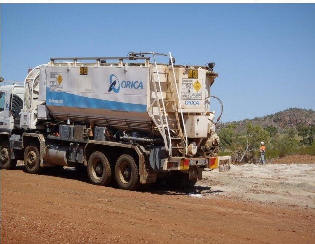
Figure 3: Charging Blast Holes with bulk explosives and Priming.
