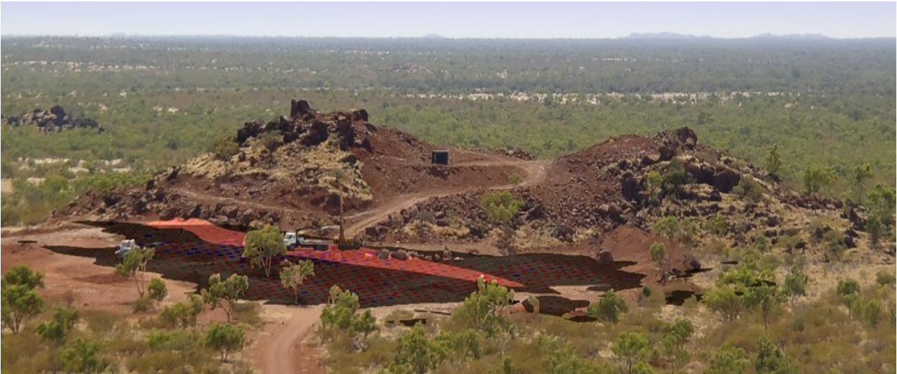
Figure 2: Wilgar Twin-hills, as viewed from the top of the nearby Breccia Hill, with indicative outline of currently identified Wilgar mineralisation (dark and light shading). The dark shaded area is the shallow mineralised outline identified to date from bedrock drilling. The light-red shaded area is the interpreted sub-cropping high-grade zone which is up to 15m wide. Mineralisation remains open along strike to the west, north, and at depth. Uranium mineralisation has not previously been targeted.
