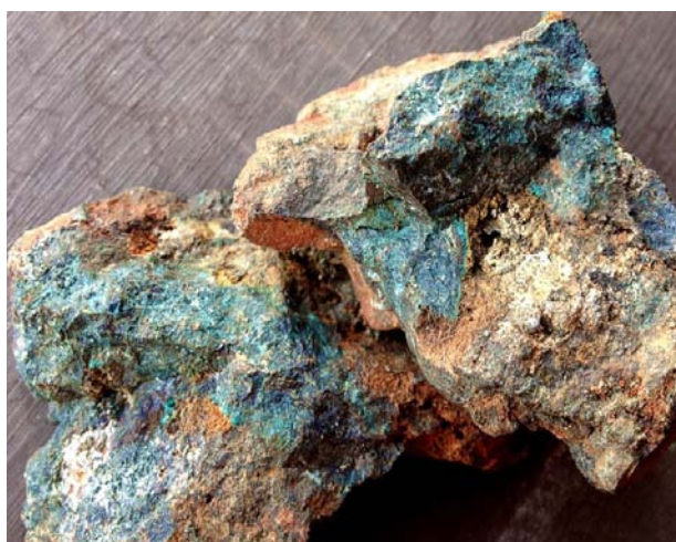
Figure 7: Sample of high-grade copper mineralisation taken from outcrop uncovered during earthworks; Malachite, azurite, chalcocite, chalcopyrite, bornite and fine-grain native copper within silicified siltstone breccia and magnetite.
