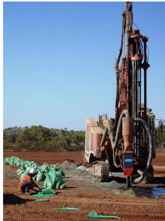
Figure 49: The green-grey/olive coloured high-grade copper-rich ore is easily identified against the red-coloured, iron-rich gangue (waste) material left on surface after completion of the bedrock holes.
