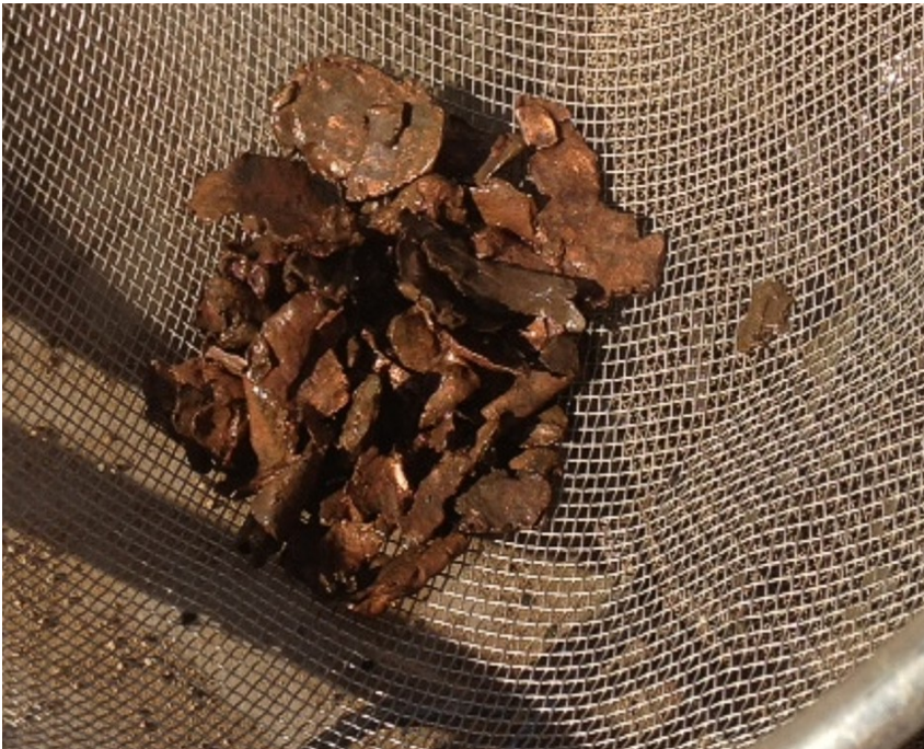
Figure 50: Native copper flattened by the bedrock drill, recovered from LMOX703, from 18-25m, in an area not previously identified to host native copper. Many of the pieces are larger than 20mm in size.
