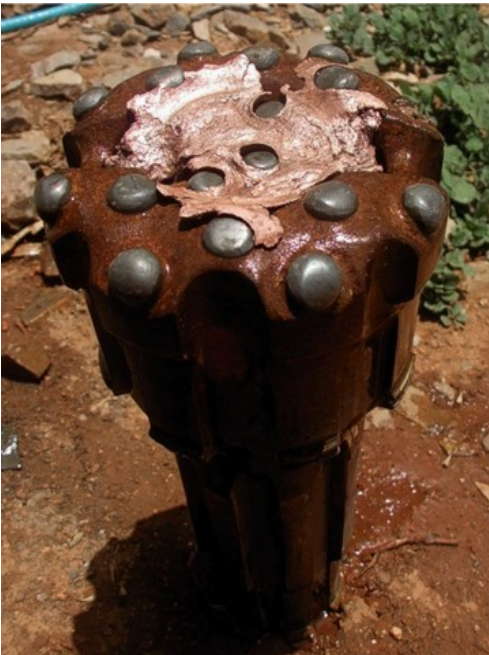
Figure 48: Example of large native copper nugget, possibly encountered in soft clay or friable oxide material and unable to return up the small (20mm) sample return holes at the end of the RC bit. Left; the remaining middle section appears to have been “stamped” out of a larger solid copper nugget that has been flattened, then cut through by the bit and right; underside of the copper “stamp” showing how the metal was pushed into the two 20mm sample return holes (top right & bottom left) and was unable to return to surface.
