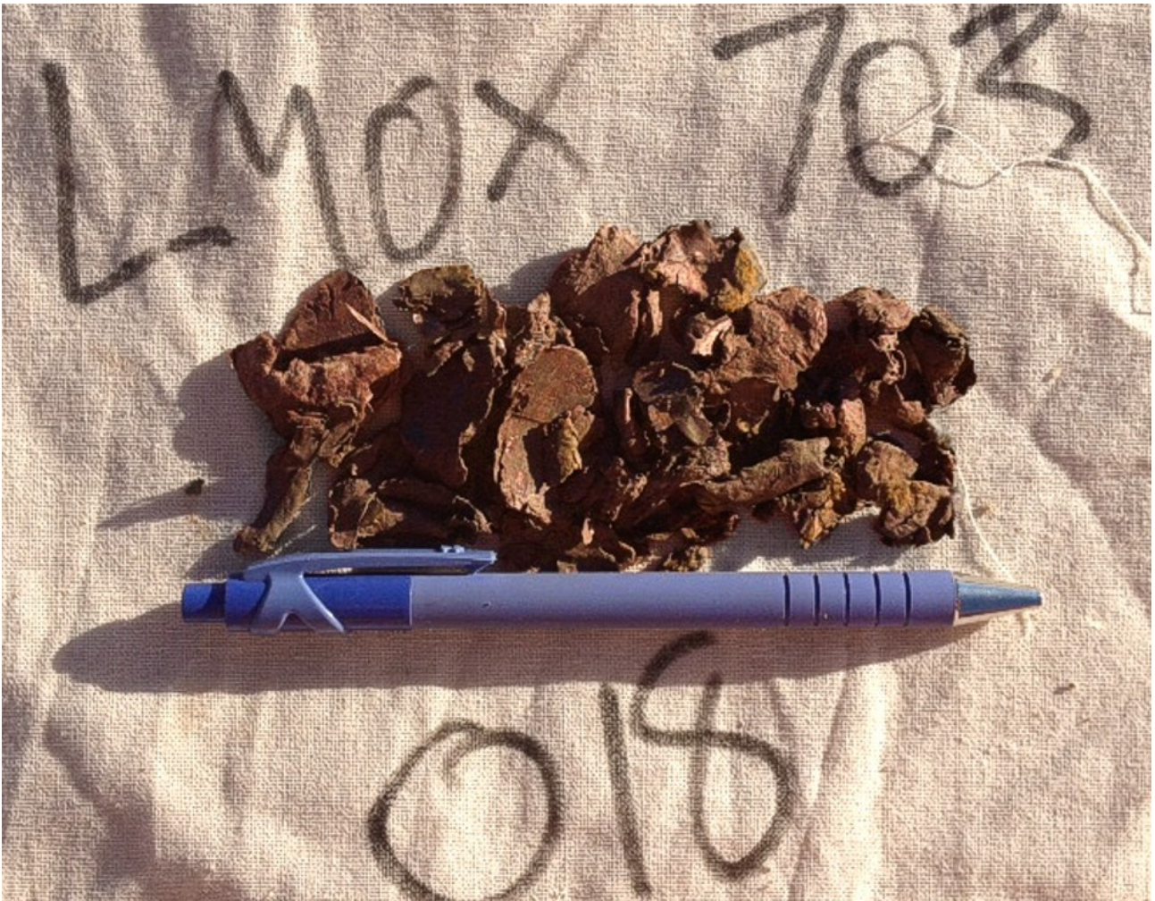
Figure 42: Native copper flattened by the bedrock drill, recovered from LMOX703, from 18-25m, in an area not previously identified to host native copper.
