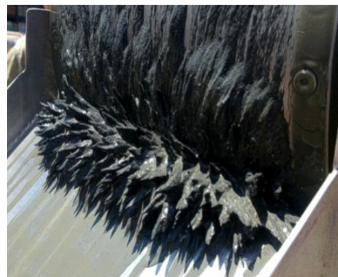
Figure 11: Various products from bulk-sample test-work (from top to bottom & left to right); large native copper nuggets (+40mm); smaller native copper nuggets (+4mm-40mm); light-grey flotation froth (primary circuit - chalcocite); yellow flotation froth (primary circuit - chalcopyrite); chalcopyrite/cobaltic pyrite concentrate and; magnetite separation of magnetite.
