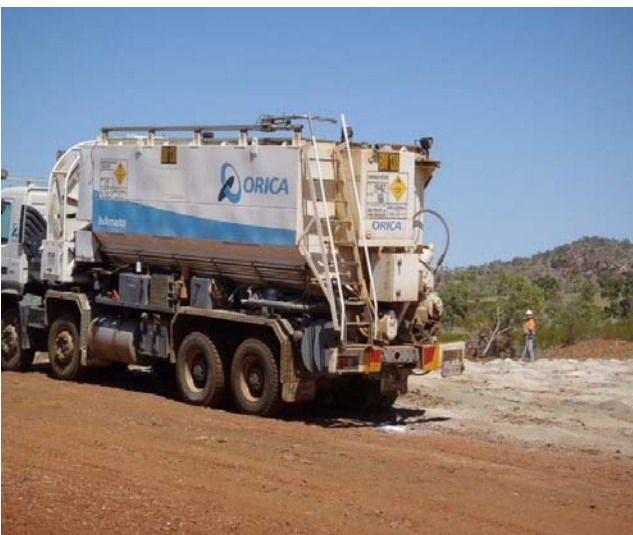
Figure 10: Charging Blast Holes with bulk explosives and Priming.
