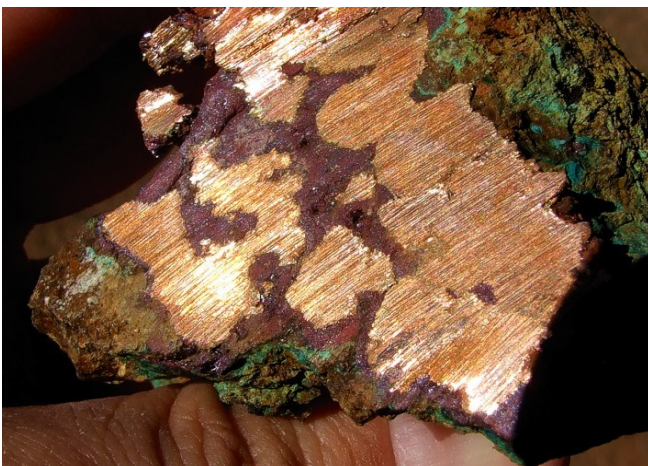
Figure 44: Native copper nugget cut with diamond saw, recovered at 5m depth from test costean excavated earlier in the year over Las Minerale. The area defined as the “native copper domain” within the current resource block model, did not identify native copper to be present at the depths being targeted in the costean.
