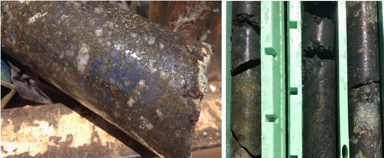
Figure 54: Example of high-grade drill core intersected in DODDH448 at Fairfield. Massive and semi-massive chalcocite (chalcocite contains 79.9% copper metal), and minor chalcopyrite (chalcopyrite contains 34.6% copper metal), bornite (bornite contains 63.3% copper metal) and pyrite (cobalt is associated with pyrite at Fairfield). Left approx. 83m, right approx. 81-84m...announced subsequent to quarter end.
