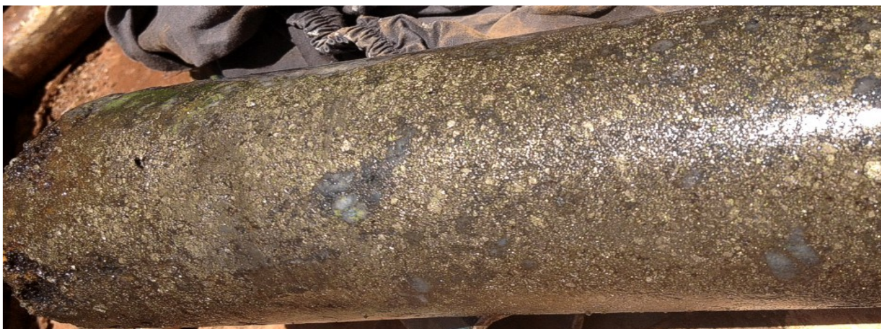
Figure 4: Example of high-grade drill core intersected in DODDH448 at Fairfield at approximately 83.2m which assayed 7.95% CuEq over 1m. Massive and semi-massive chalcopyrite and pyrite and minor chalcocite and bornite. Chalcocite contains 79.9% copper metal, chalcopyrite contains 34.6% copper metal, bornite contains 63.3% copper metal. Cobalt is associated with pyrite at Fairfield.
