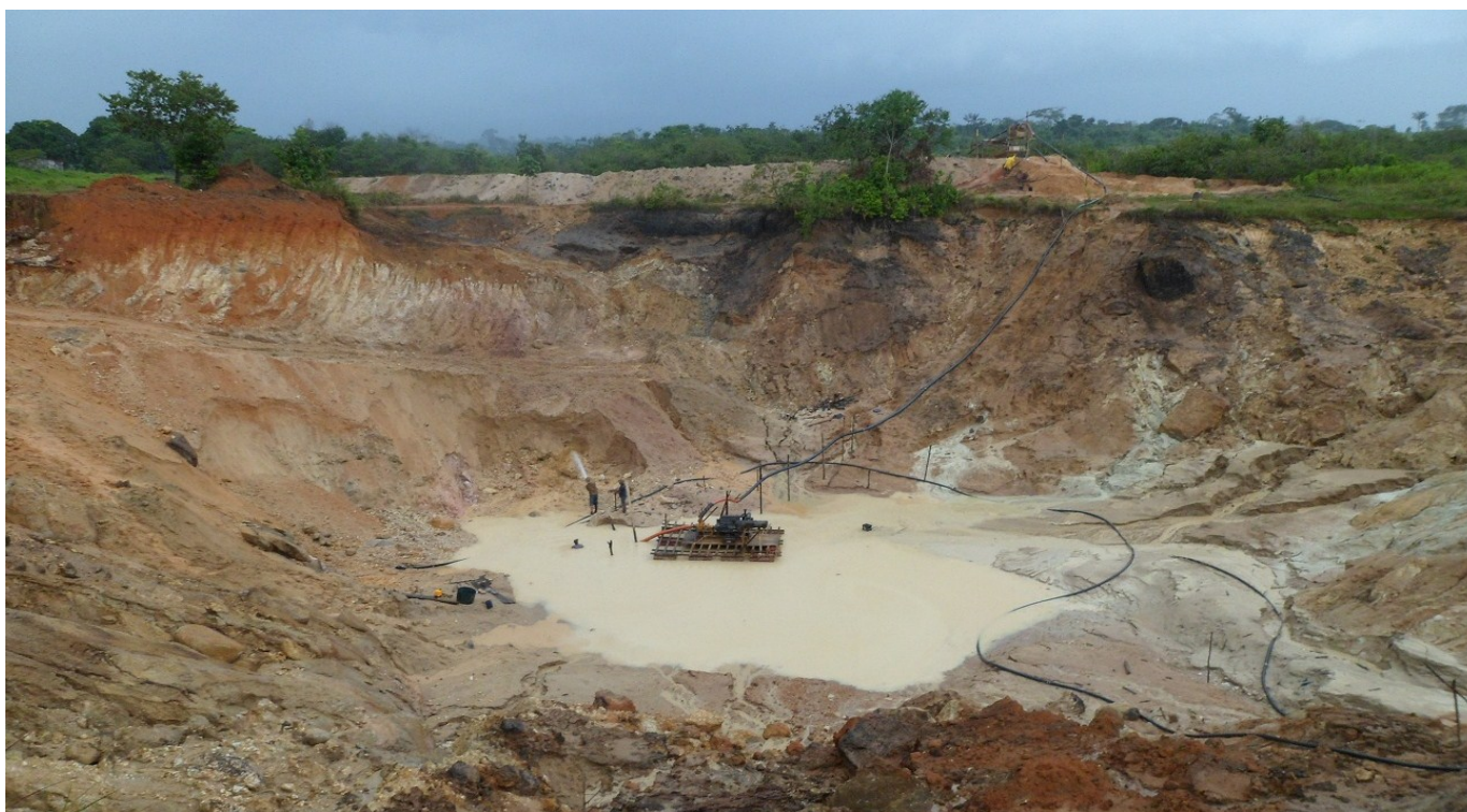
Figure 3: Tambaqui west pit undergoing dewatering.
