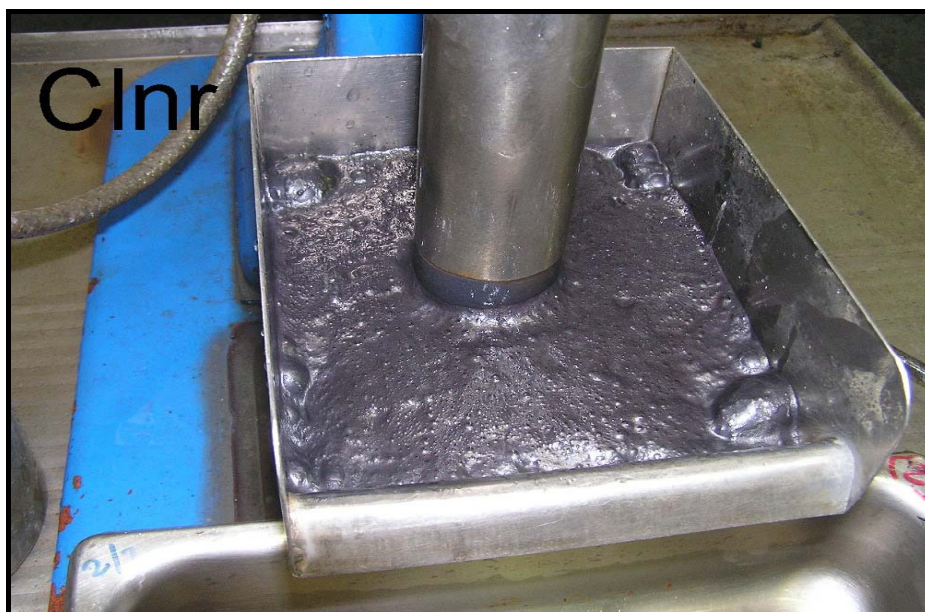
Preliminary flotation concentrate tests – the silver coloured bornite can be clearly seen
