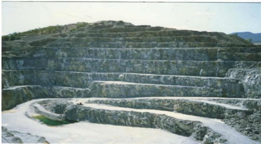
Figure 3. The open-pit at Mt Carbine in 1986. The pit will be pushed back to provide ore for the proposed second stage of development at Mt Carbine.
