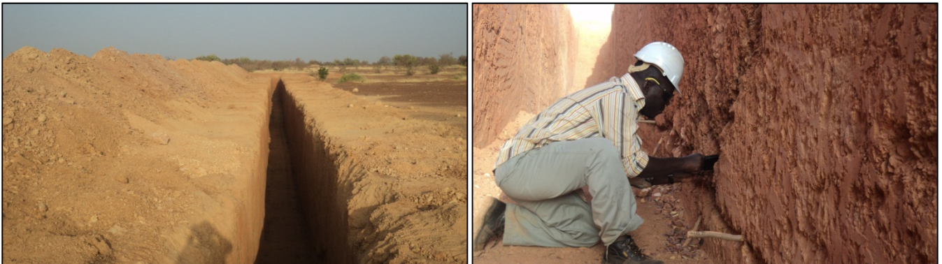
Figure 5: Trench sampling and mapping at the Foufaka Prospect on the Kandy Permit.
