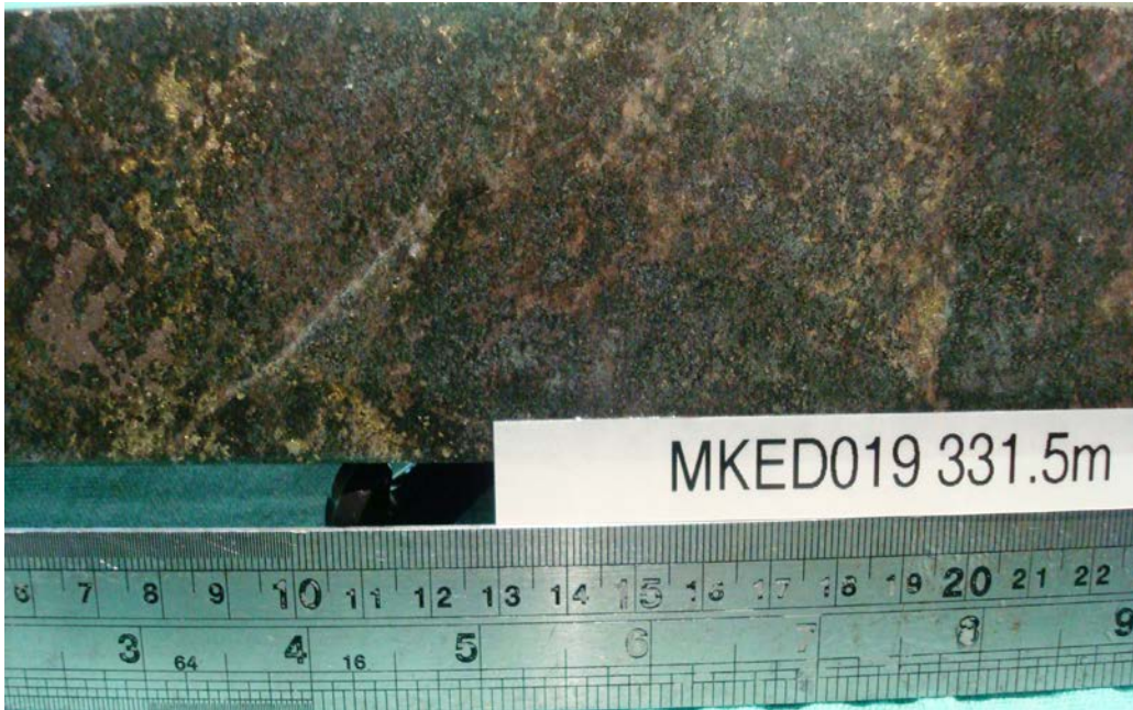
Photo 1: MKED019, ~335 metres - Phyrrhotite+pyrite+chalcopyrite mineralisation. Assays returned for interval = 1m @ 1.17% copper, 214ppm cobalt and 0.04 g/t gold (335m – 336m).
