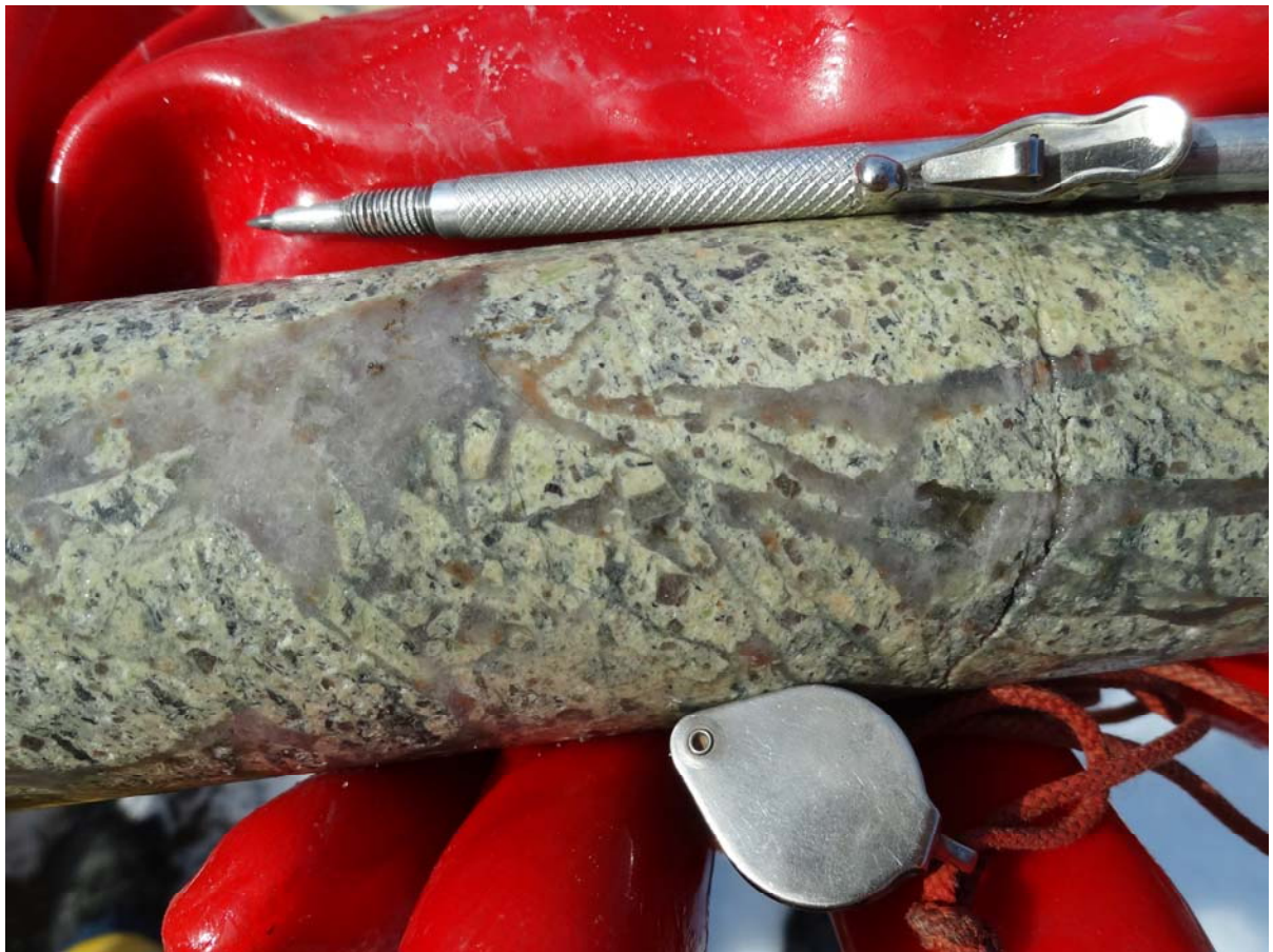
Vein quartz, disseminated pyrite and galena in clay altered rock, SM-12-02, 82.3m
