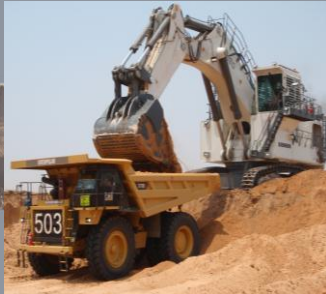
Liebherr 9350 Excavator and Caterpillar dump truck
