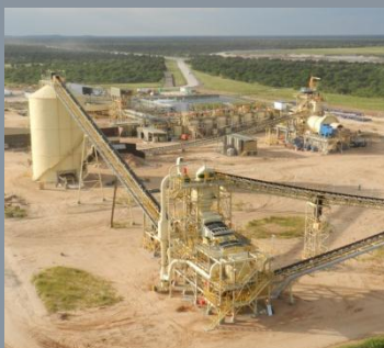
Screen plant and crushed ore bin
