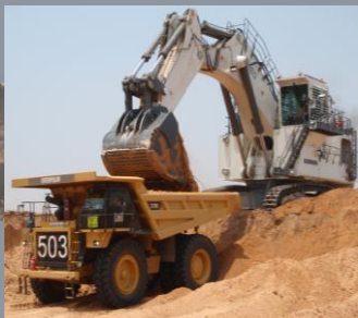
Liebherr 9350 Excavator and Caterpillar dump truck
