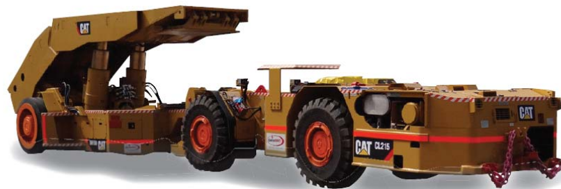
15 tonne loader with chock trailer
