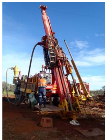
Versadrill RC rig in use at Sabbath
