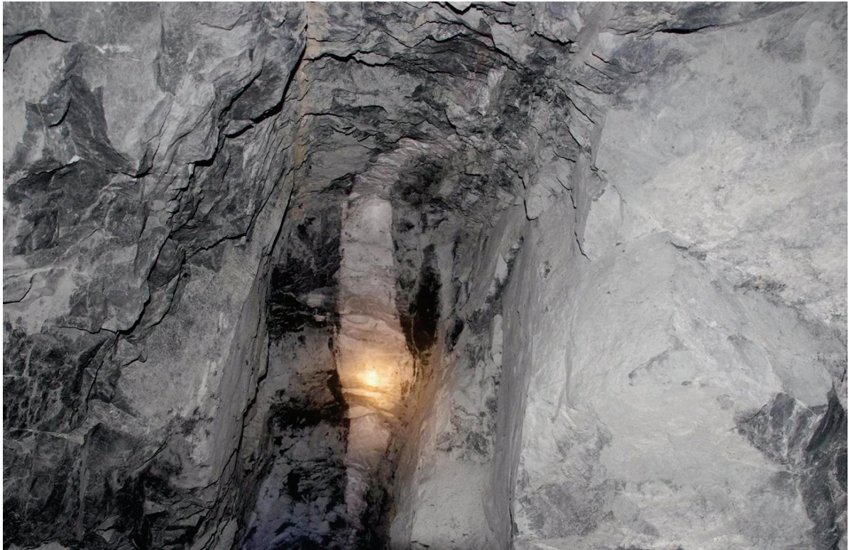
Figure 3 The gold bearing quartz reef in one of the stopes level 2 south drive.
