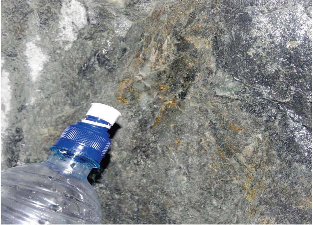
Figure 2 Gold and sulphide mineralisation on side of stope near end of level 1 north drive
