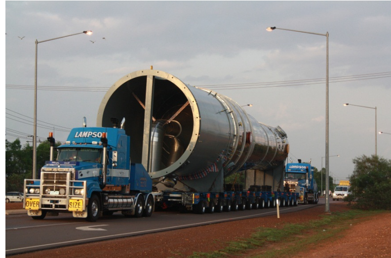
Transportation of evaporator vessel from Darwin Port to Ranger mine
