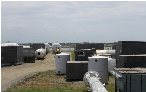
Cold-boxes and ancillary equipment for the Sengkang LNG Project arriving on site in Sengkang, Indonesia
