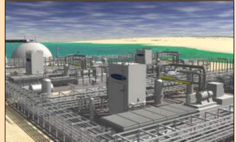
Cold Box and Compressor
