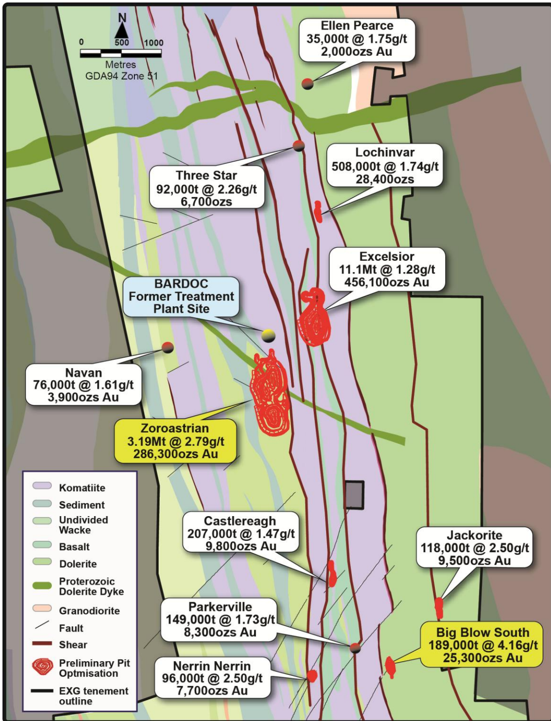
Figure 4. Kalgoorlie North Gold Project – Central Resource Area Geological Plan (showing current resource areas and preliminary pit optimisation shells with resources quoted at 0.6 and 3.0g/t Au lower cut-offs )
