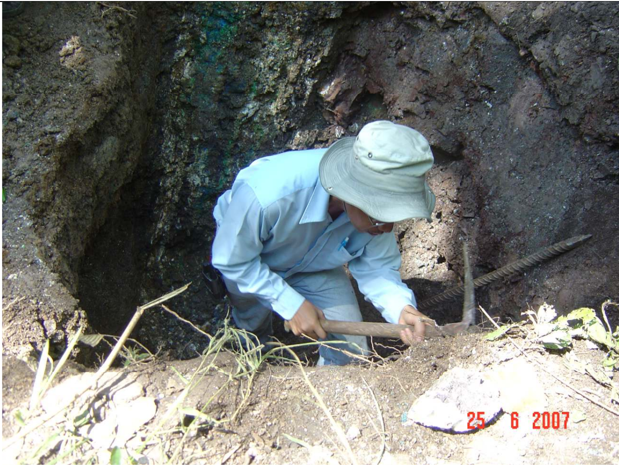
FIGURE 13: Azurite and malachite within steeply dipping vein in costean at the Sroyang License
