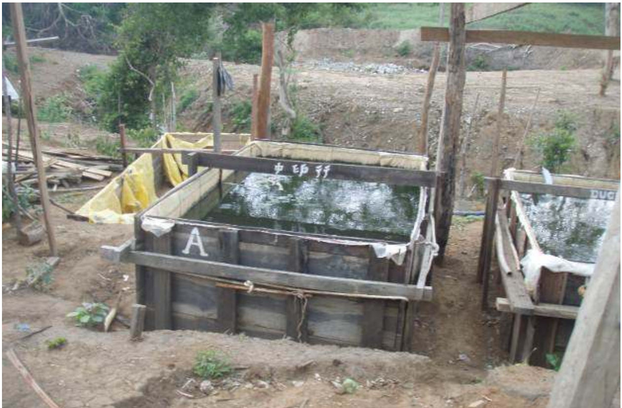
FIGURE 5: Solvent extraction vats for copper carbonate ore.
