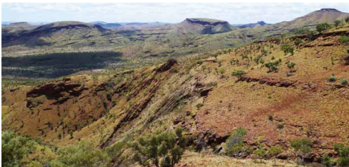
Plate 1 Photo looking east across Blackjack deposit on E47/882 Blacksmith, clearly showing near vertical BID rich structural zone in the centre foreground.
