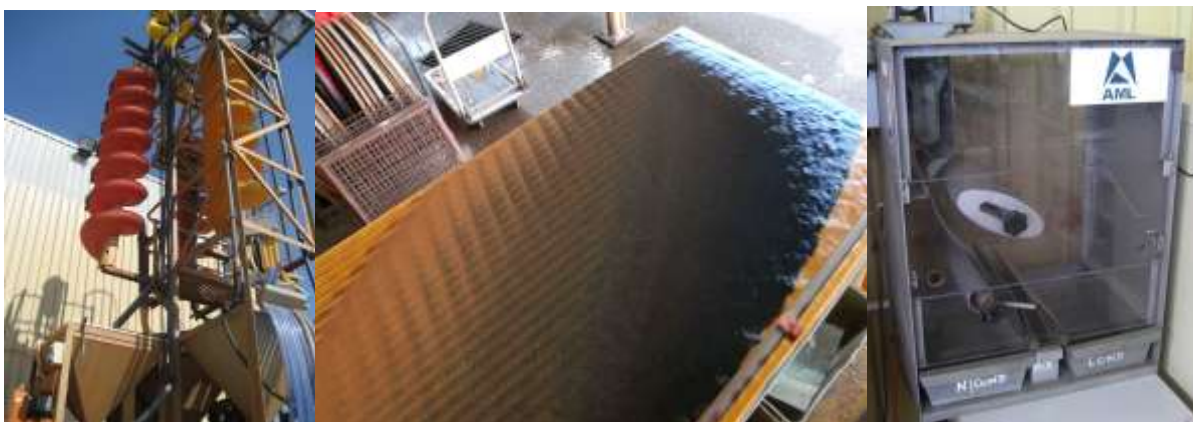
Figure 1. AML equipment used in the heavy mineral separation test work. The centre photograph shows the heavy mineral from the McLaren Deposit being separated by wet table.
