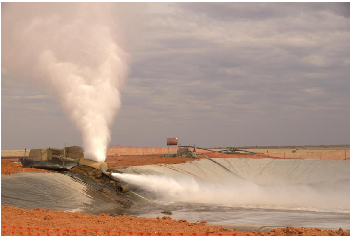
Above: Steam flowing at Habanero 4 during well clean-up program on Saturday 20 October 2012.
